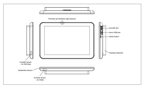
Figure 2. HD Display 3.0 Components
