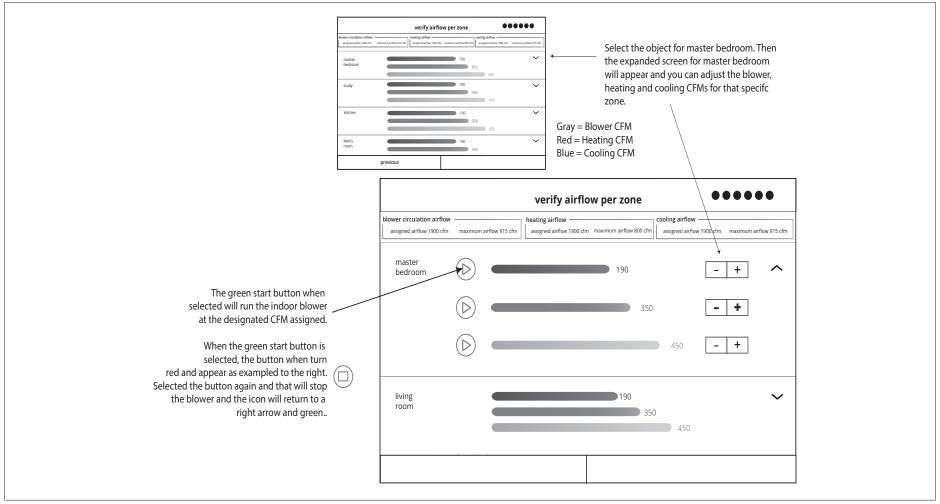
Figure 18. Verify Airflow Per Zone Screen
