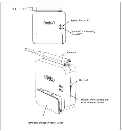
Figure 1. Smart Hub Indicators and External Components
