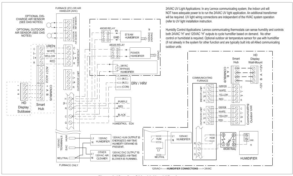
Figure 9. iComfort S30 with Humidifier Accessory
