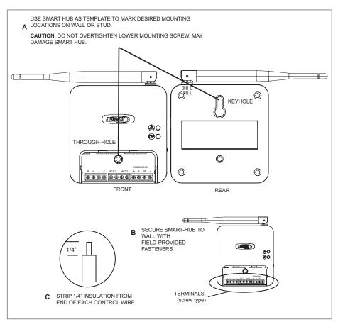
Figure 14. Smart Hub Installation
