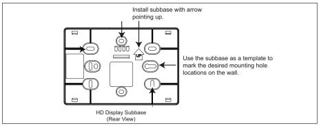
Drill 3/16" (5 mm) holes at marked locations on the wall for anchors. Then
