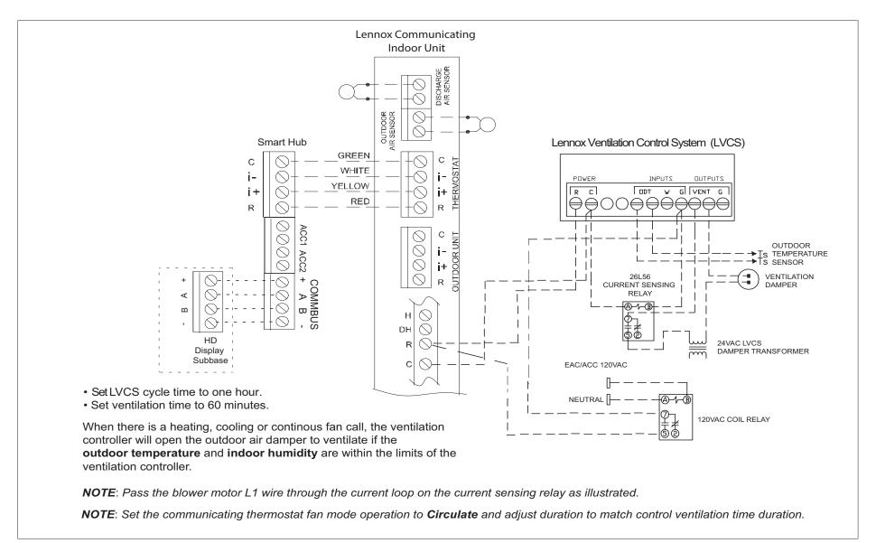
Figure 10. iComfort S30, Lennox Ventilation Control System (LVCS), Current Sensing Relay, 120VAC Coil Relay, Damper Transformer, Ventilation Dampers and Communicating Indoor Unit (using Non-Communicating Terminals)
