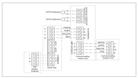
Figure 4. iComfort S30 with Lennox Communicating Indoor and Outdoor Units
