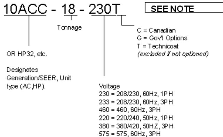
Note: Revision level will appear in the revision block below the model number on Nameplates. Bill of Material spreadsheets will show the revision level at the end of the model number.
