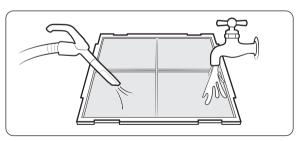
Clean the air filter with a vacuum cleaner or soft brush. If dust is too heavy, then rinse it with running water and dry it in a ventilated area.
