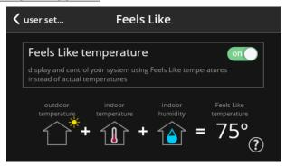
Accurately controls temperature in the home by determining the "feels like" temperature based on outdoor temperature, indoor temperature plus indoor relative humidity.
