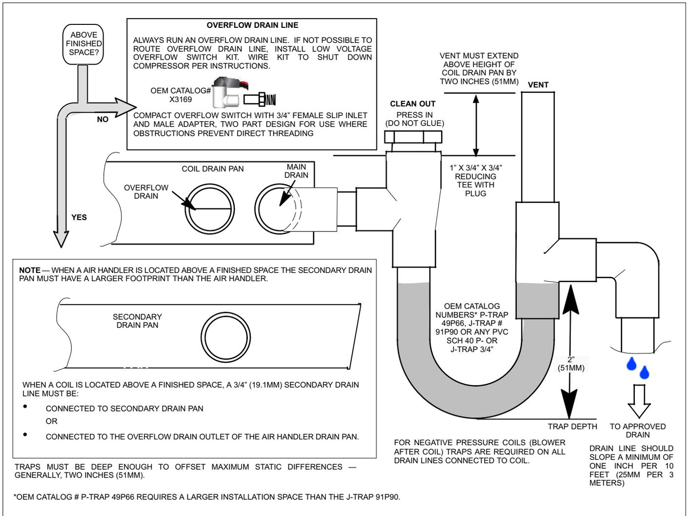
**Figure 4. Typical Main and Overflow Drain Installations**
