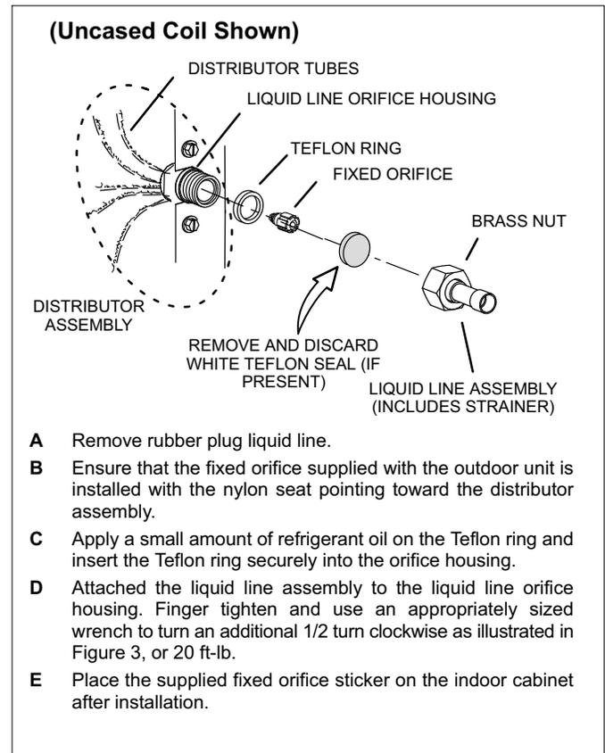
**Figure 2. Typical Fixed Orifice Metering Device Installation Procedure**
