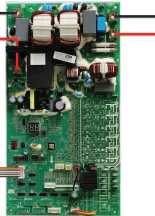
(Single Phase, Gas Cooler) IPM Board
