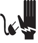
Electric shock hazard. Can cause injury or death. Before attempting to perform any service or maintenance, turn the electrical power to unit OFF at disconnect switch(es). Unit may have multiple power supplies.
