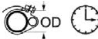
**REMARQUE - NE JAMAIS MONTER LE BULBE DE DÉTECTION EN DESSOUS DE LA CONDUITE.**
