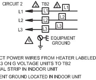
**FIELD WIRING FOR UNITS WITH CIRCUIT BREAKERS**
