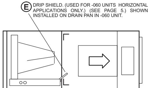
**E** DRIP SHIELD. (USED FOR -060 UNITS HORIZONTAL APPLICATIONS ONLY.) (SEE PAGE 5.) SHOWN INSTALLED ON DRAIN PAN IN -060 UNIT.
