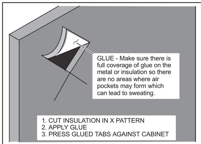
**FIGURE 13. Repairing Insulation**
