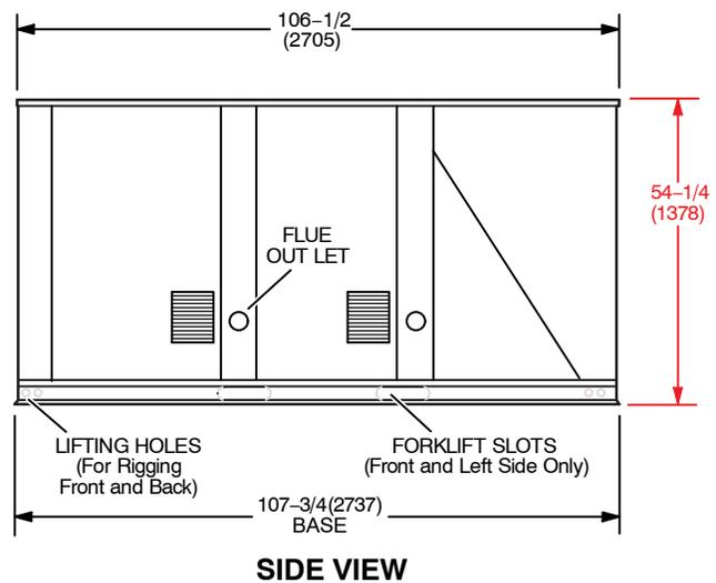
**KG/KC 240S, 300S DIMENSIONS - Electric heat section shown**
