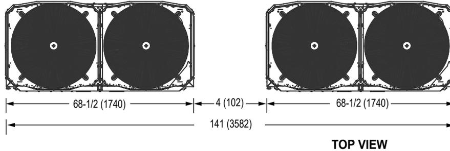
**NOTE - All the outdoor units manifolded together should be installed at the same elevation.**
