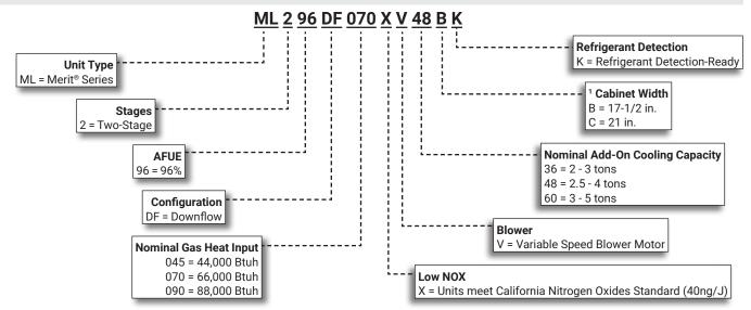
1 1 Downflow indoor coils with the same letter designation will physically match the furnace supply air opening.
