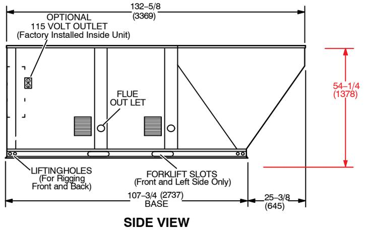
**LGT/LCT 240H & 300S Unit Dimensions - Inches (mm)-Gas Heat Section Shown**
