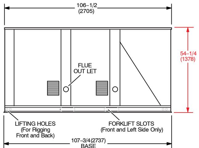
**LGT/LCT180H, 210H Unit Dimensions - Inches (mm) - Gas Heat Section Shown**
