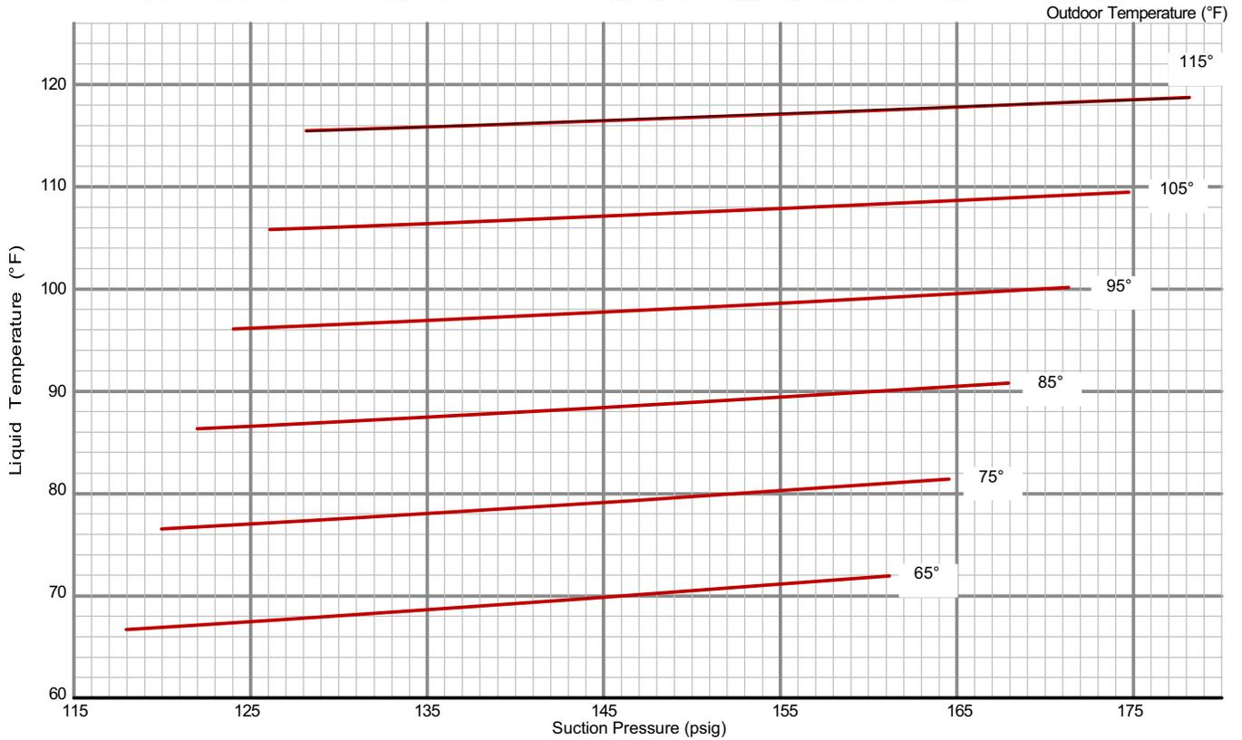
**210 CHARGING CURVE CIRCUIT 2 - NO REHEAT - ALL-ALUMINUM COIL - 581090-01**
