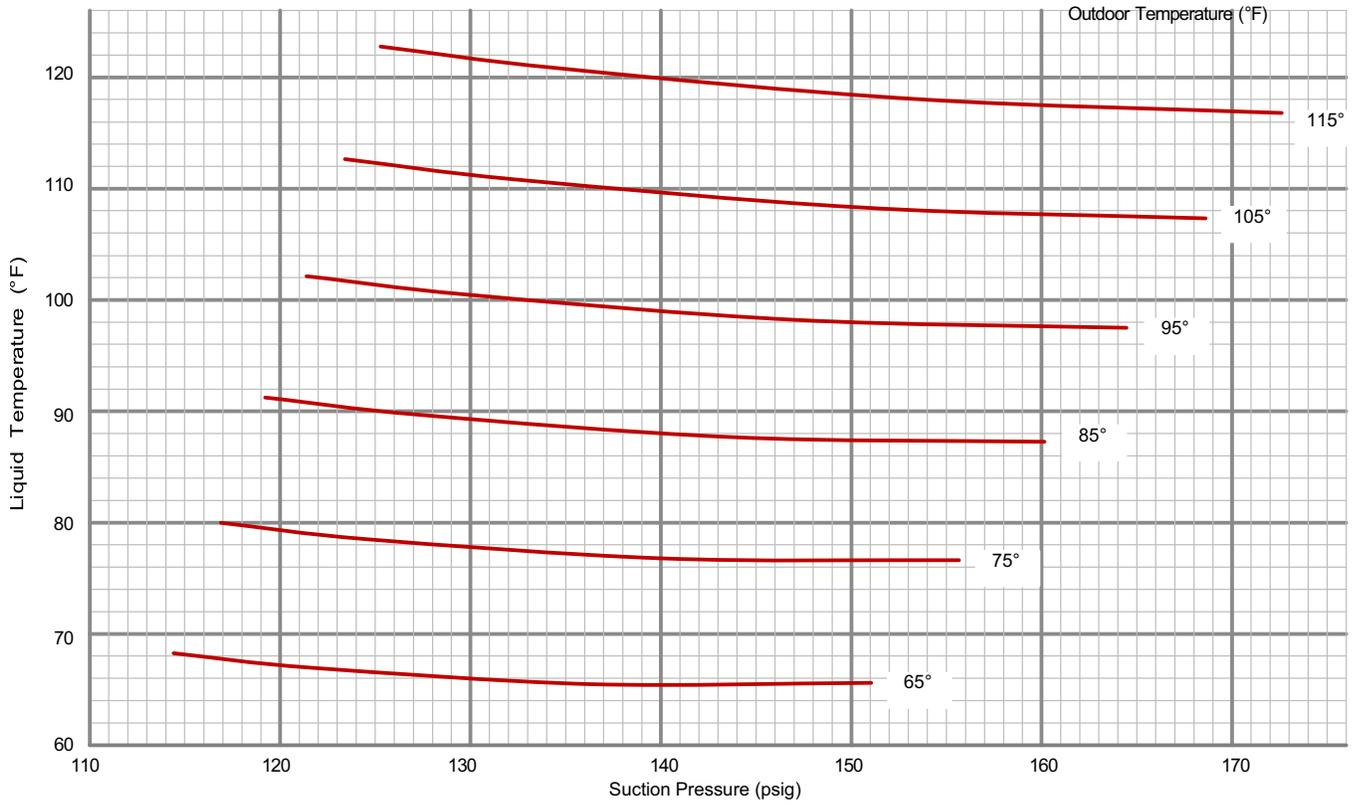
**240 CHARGING CURVE CIRCUIT 3 - REHEAT - ALL-ALUMINUM COIL - 581096-01**
