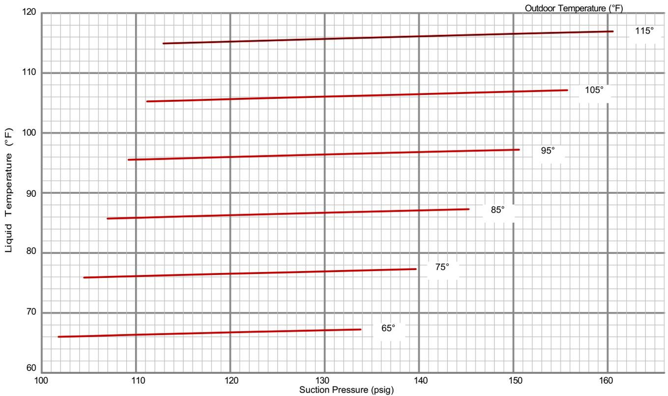
**180 CHARGING CURVE CIRCUIT 2 - NO REHEAT - ALL-ALUMINUM COIL - 581086-01a**
