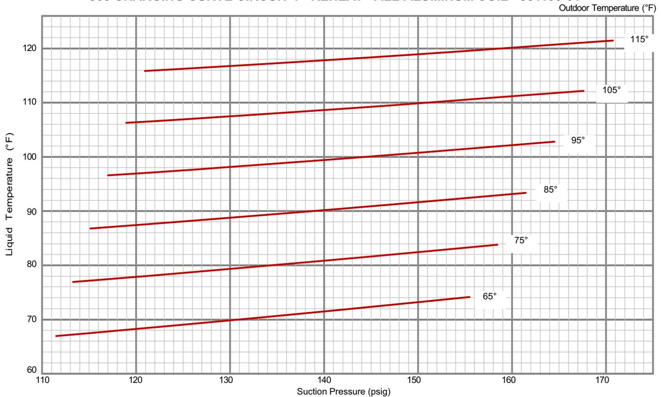
**300 CHARGING CURVE CIRCUIT 2 - REHEAT - ALL-ALUMINUM COIL - 581100-01**
