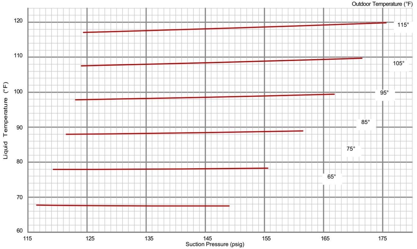
**240 CHARGING CURVE CIRCUIT 3 - NO REHEAT - ALL-ALUMINUM COIL - 581094-01**
