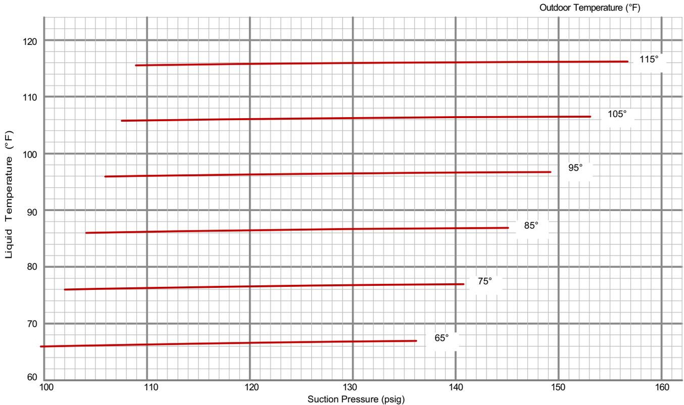
**180 CHARGING CURVE CIRCUIT 2 - REHEAT - ALL-ALUMINUM COIL - 581088-01**
