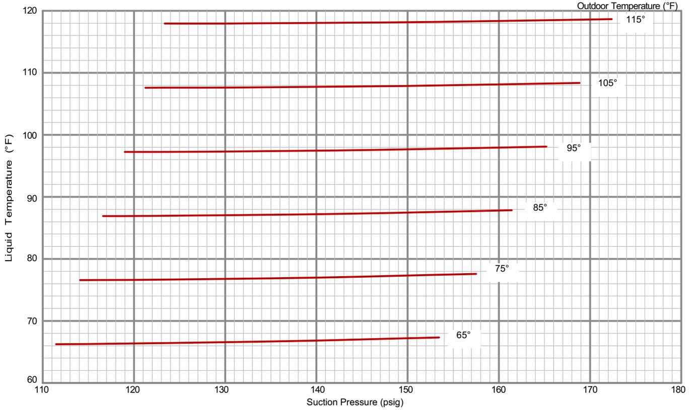
**300 CHARGING CURVE CIRCUIT 3 - REHEAT - ALL-ALUMINUM COIL - 581100-01**
