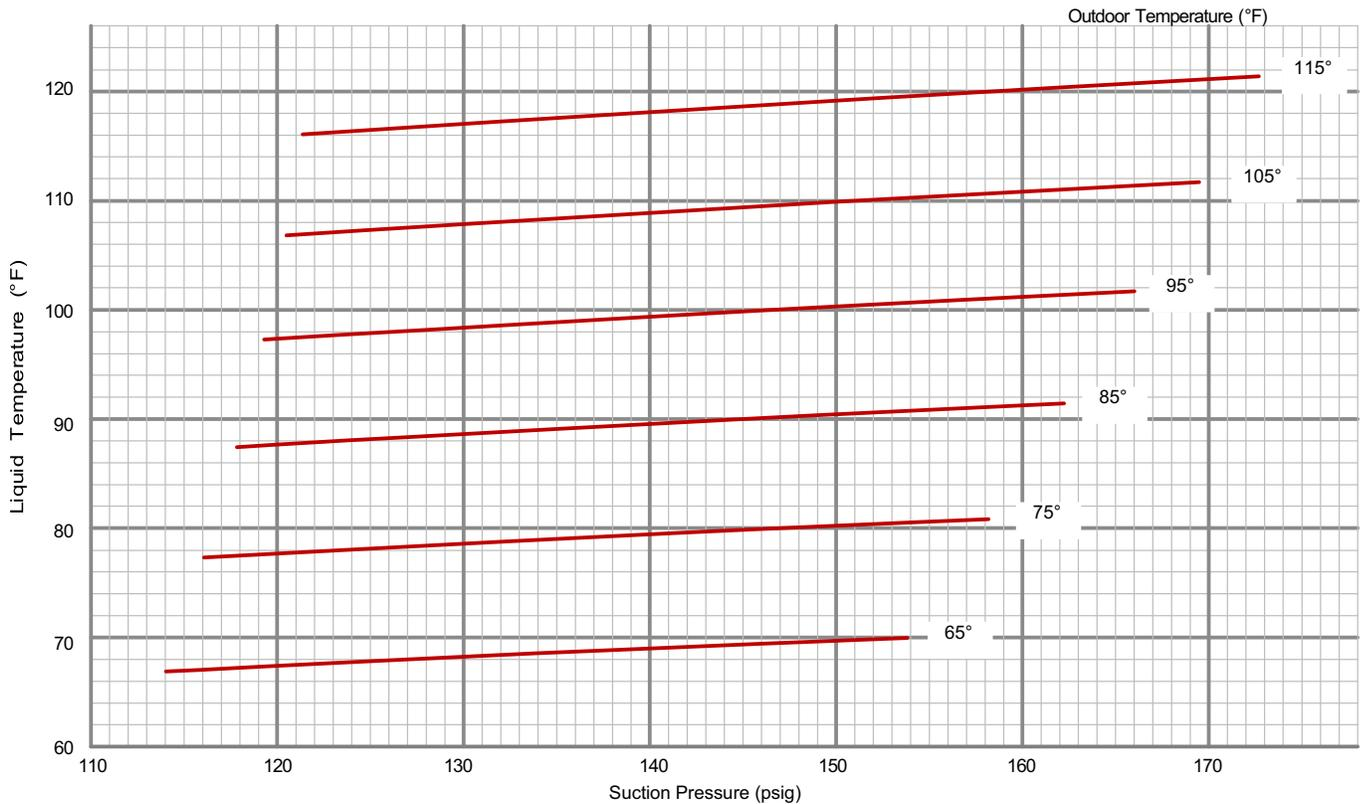
**240 CHARGING CURVE CIRCUIT 2 - NO REHEAT - ALL-ALUMINUM COIL - 581094-01**
