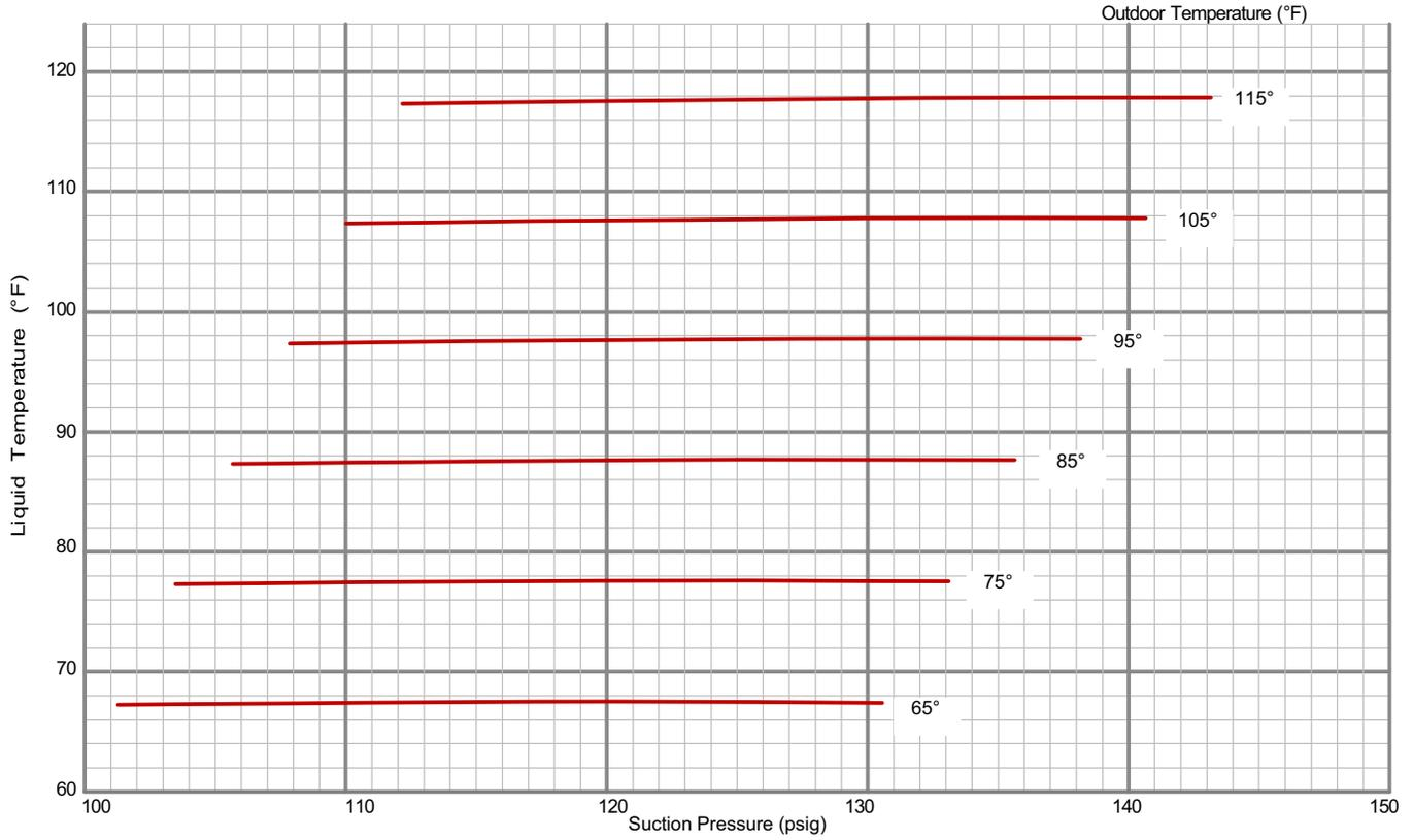
**180 CHARGING CURVE CIRCUIT 3 - NO REHEAT - ALL-ALUMINUM COIL - 581086-01a**
