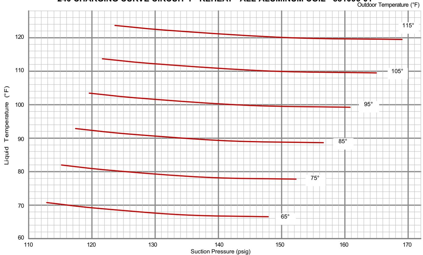
**240 CHARGING CURVE CIRCUIT 2 - REHEAT - ALL-ALUMINUM COIL - 581096-01**
