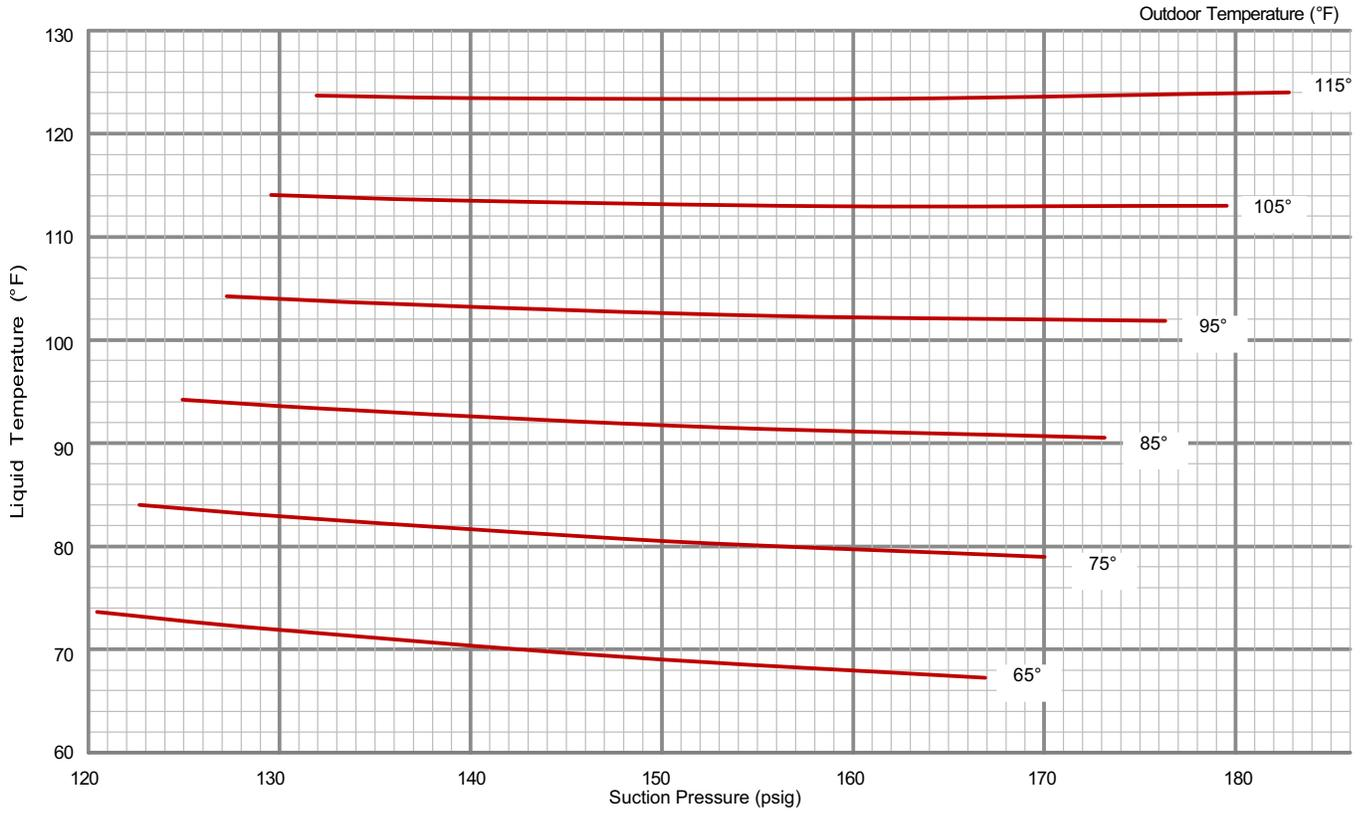
**210 CHARGING CURVE CIRCUIT 3 - REHEAT - ALL-ALUMINUM COIL - 581092-01**
