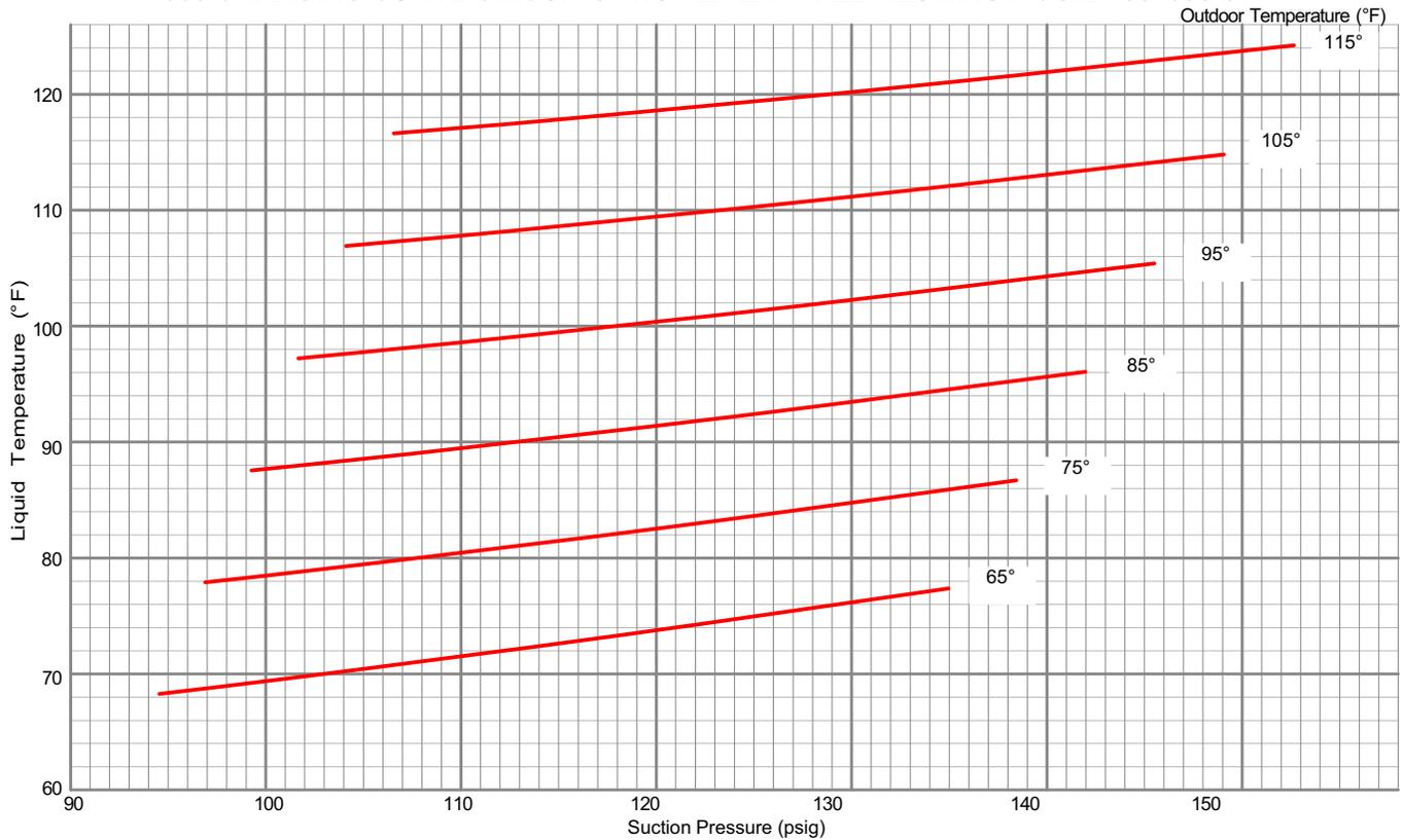
300 CHARGING CURVE CIRCUIT 4 - NO REHEAT - ALL-ALUMINUM COIL - 581098-01
