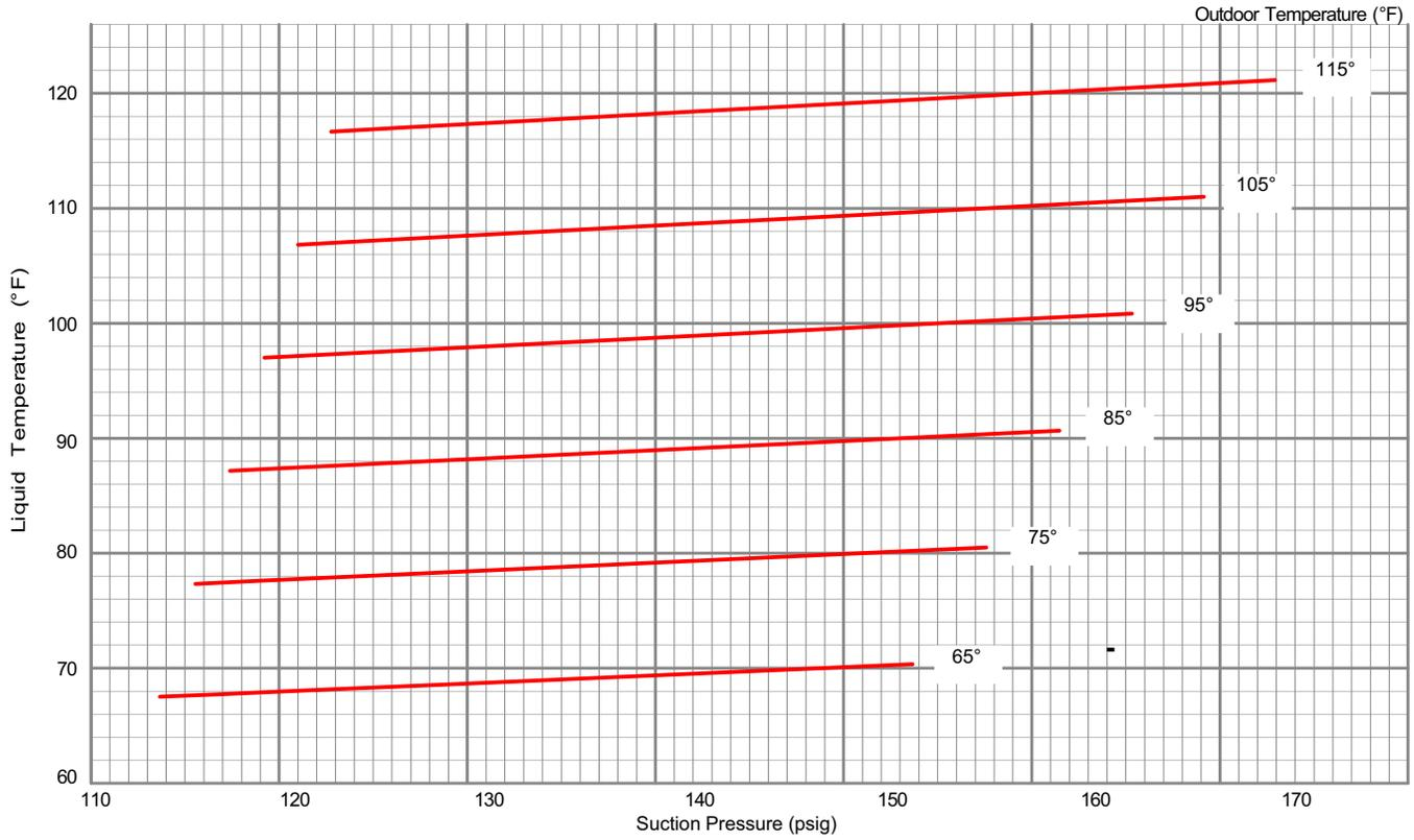
**300 CHARGING CURVE CIRCUIT 3 - NO REHEAT - ALL-ALUMINUM COIL - 581098-01**
