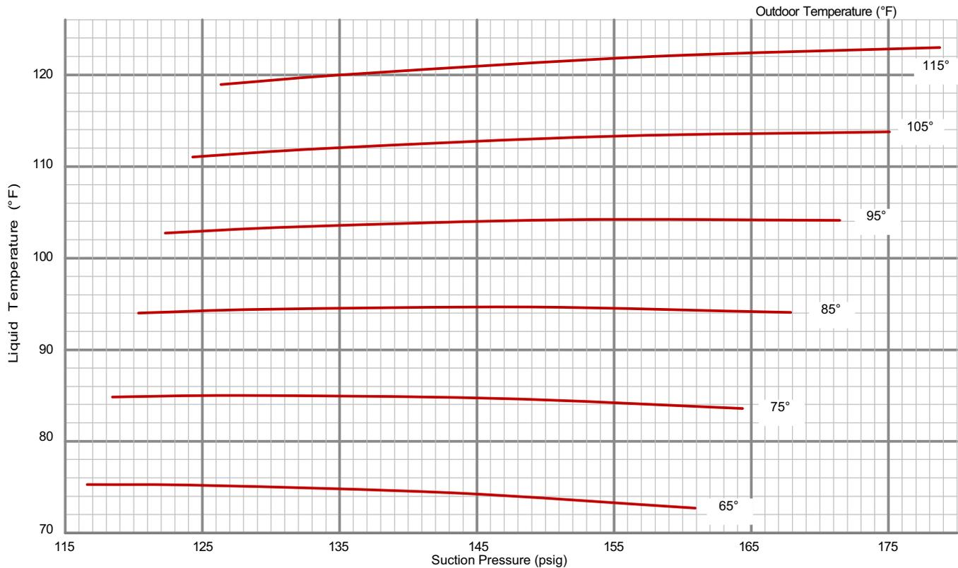
**210 CHARGING CURVE CIRCUIT 2 - REHEAT - ALL-ALUMINUM COIL - 581092-01**
