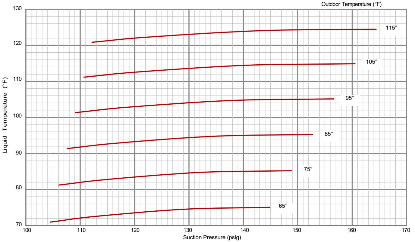
**180 CHARGING CURVE CIRCUIT 3 - REHEAT - ALL-ALUMINUM COIL - 581088-01**
