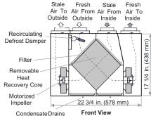
Note: Front clearance of 25 in. (635 mm) is recommended for servicing unit. All ducts use 5 in. (125 mm) oval collars, balancing dampers are located on all collars.
