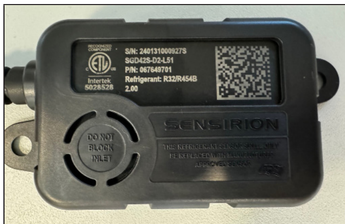
FIGURE 22. Example of Clear, Unobstructed Sensor Inlet
