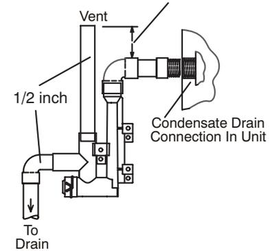
Drain Trap Assembly with 3/4 inch Piping
