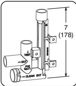
Drain Trap Assembly with 1/2 inch Piping
