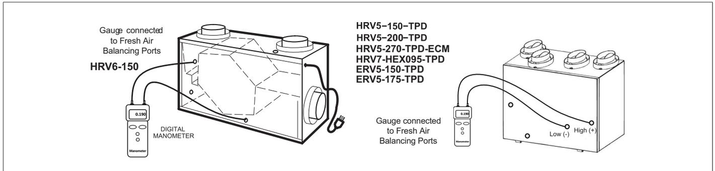
**Figure 57. Door Balancing Ports - Fresh Air**
