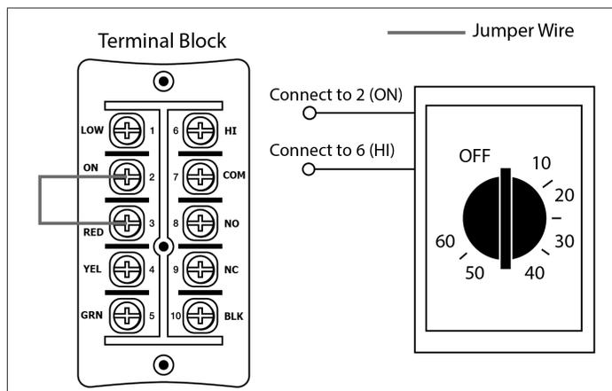
Figure 42. Mechanical Timer Installation Configuration A
