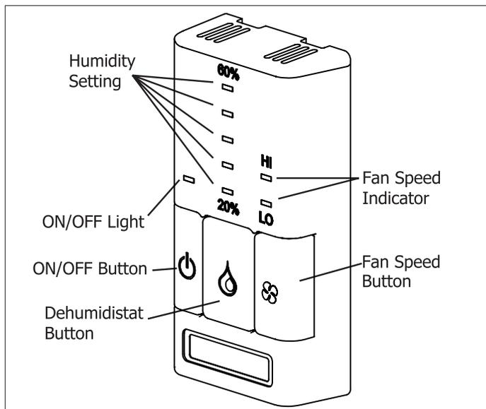
**Figure 15. H/C ERV/HRV Ventilation Push Button Control (Y8249)**
