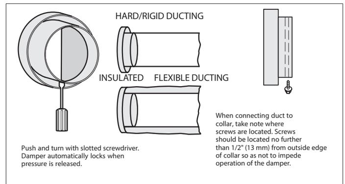
**Figure 56. Balancing Collars**
