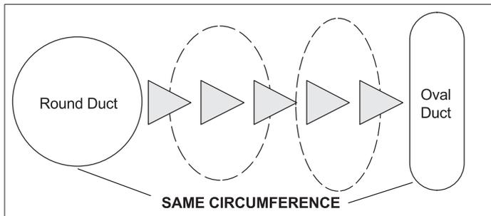
Figure 5. Shaping Ducting to Fit Oval Ports
