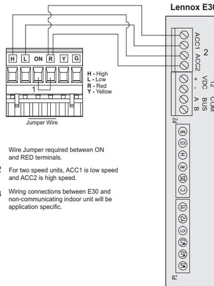
Figure 10. Lennox E30 to Ventilation Equipment Wiring Connections
