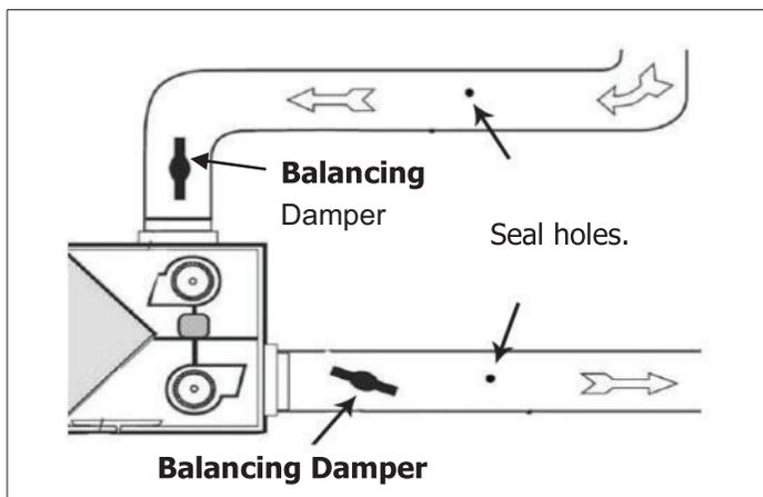
**Figure 55. Balancing Damper**
