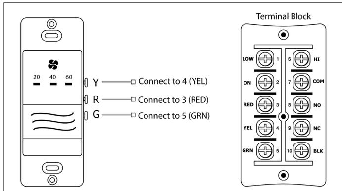
Figure 40. Wired Timer Installation (Configuration A)
