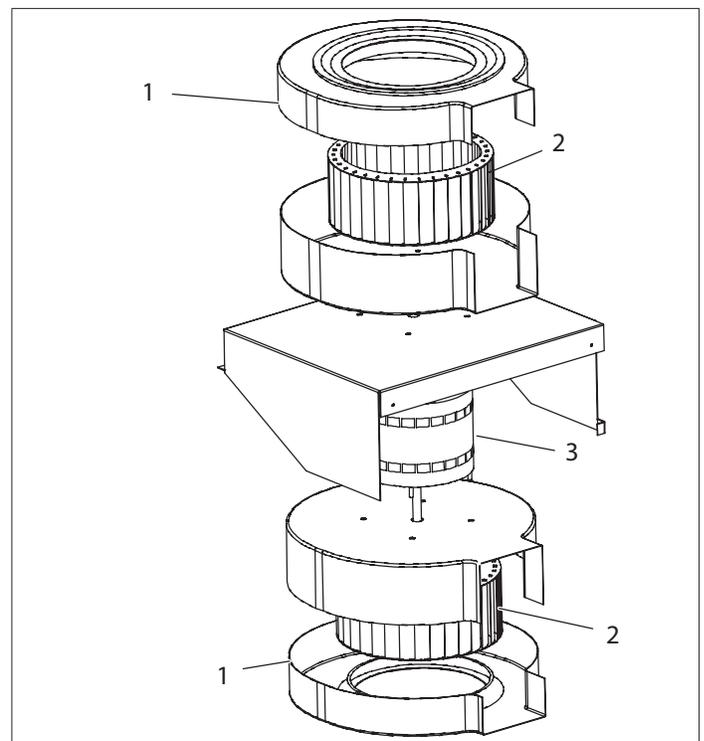
Figure 66. Replacing Motor
