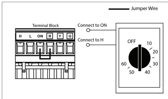
Figure 43. Mechanical Timer Installation Configuration B
