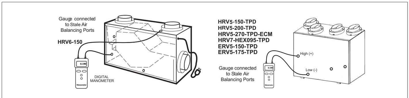
**Figure 58. Door Balancing Ports - Stale Air**
