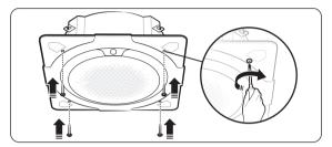
**5** Place each cover panel on a corner of the panel front. Then push the cover panel upward until it is firmly assembled to the panel front.
