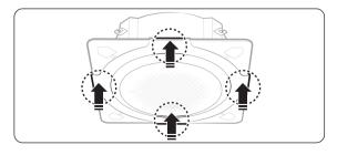
**4** Insert halfway the four screws into the four holes on the panel front. Then fasten the screws tightly until there is no gap between the ceiling and the panel front.
