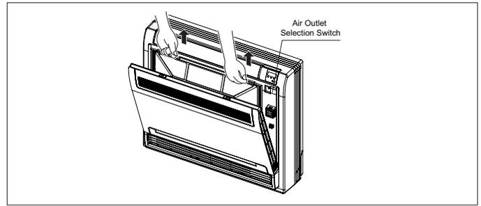
**Figure 33. Open Front Panel**
