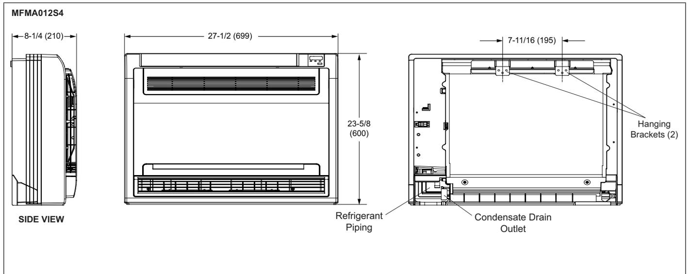
**Figure 4. MFMA Indoor Unit Dimensions - Inches (mm)**
