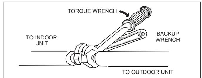
**Figure 22. Tighten Flare Nut**
