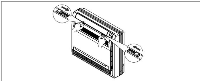
**Figure 32. Open Front Panel**
