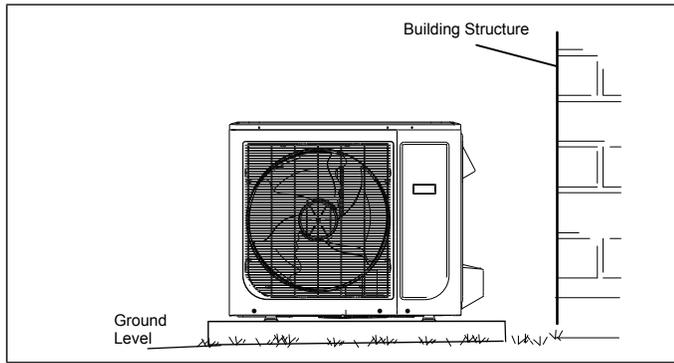
**Figure 8. Install Unit Level**
