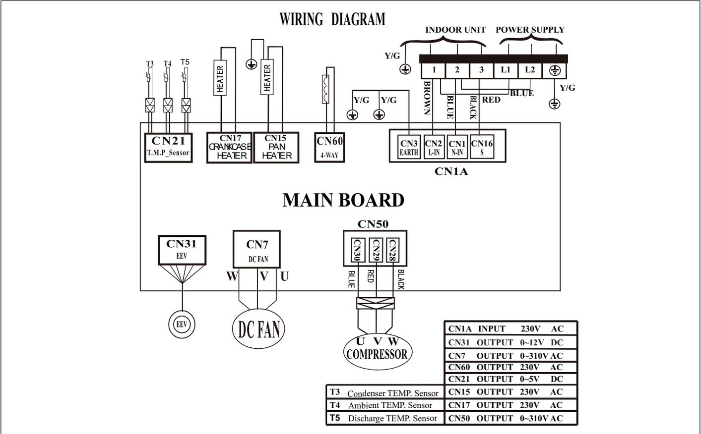
**Figure 26. 208/230V MLB012S4S-\*P Outdoor Unit Wiring Diagram**
