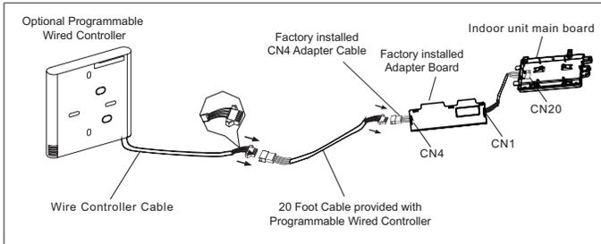
**Figure 34. Connecting Optional Programmable Wired Controller**
