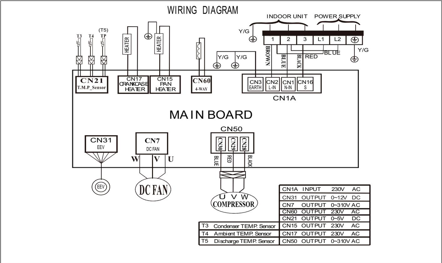
**Figure 25. 208/230V MPC012S4S-\*P Outdoor Unit Wiring Diagram**
