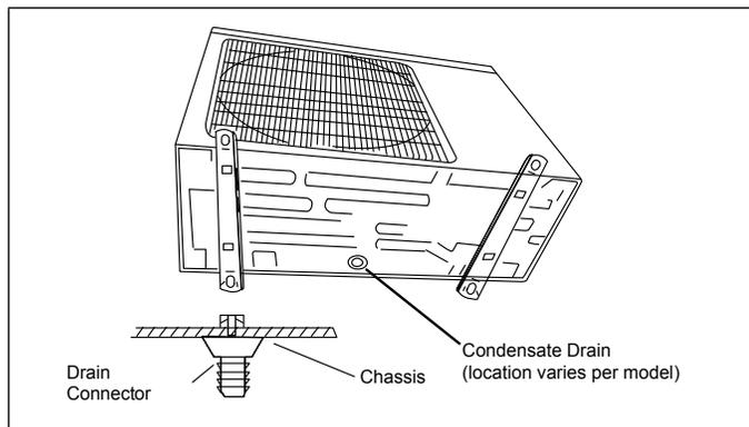
Figure 16. Condensate Drain
