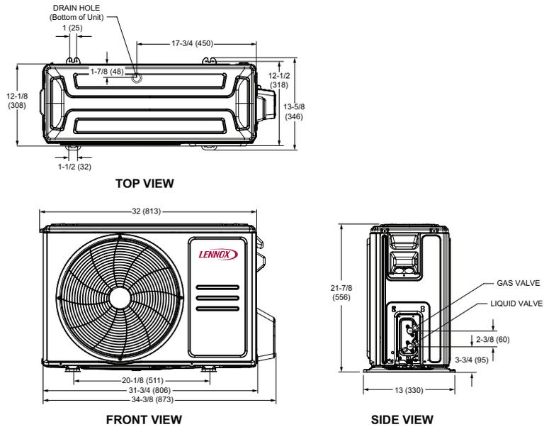
Figure 3. MLB012S4S Outdoor Unit Dimensions - Inches (mm)
