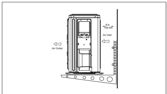
Figure 19. Securing Outdoor Unit to Brackets
