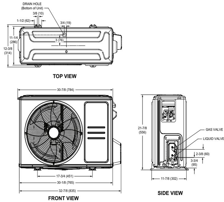
Figure 2. 208/230V - MPC012S4S Outdoor Unit Dimensions - Inches (mm)
