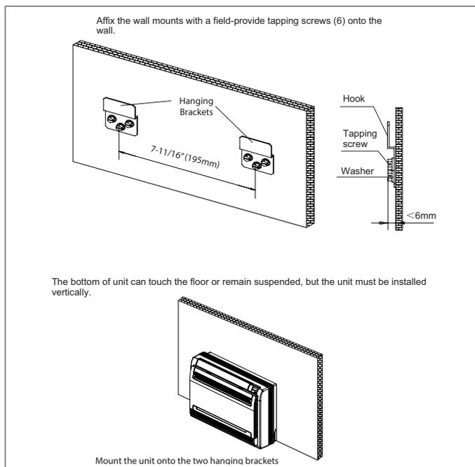
**Figure 7. Mounting Unit to Wall**
