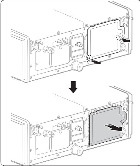
3 Disassemble two screws and remove the cover pipe.
