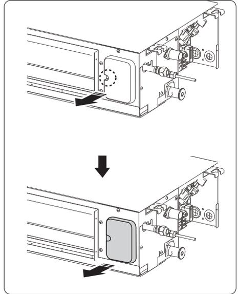
4 Pull the Wi-Fi wire through the wiring hole, and then take out the Wi-Fi module from the back side of the Cover pipe.
