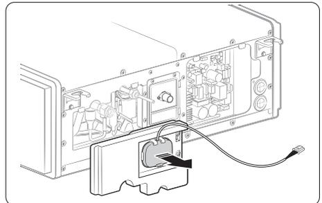
5 Connect the Wi-Fi wire connector through the wire hole .
