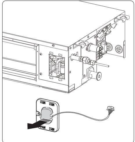
5 Connect the Wi-Fi wire connector through the wire hole.
