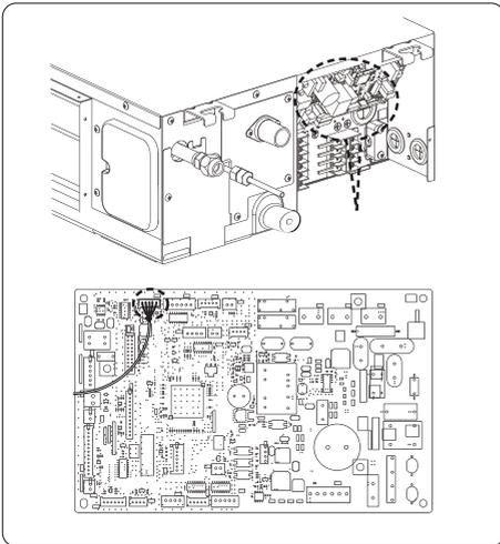
3 Remove one screw and remove the Cover case.
