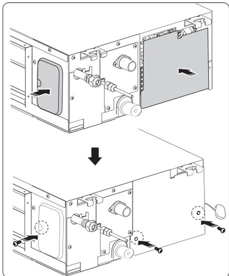
7 Fix the Wi-Fi module to the Ceiling to avoid the steel structure.
