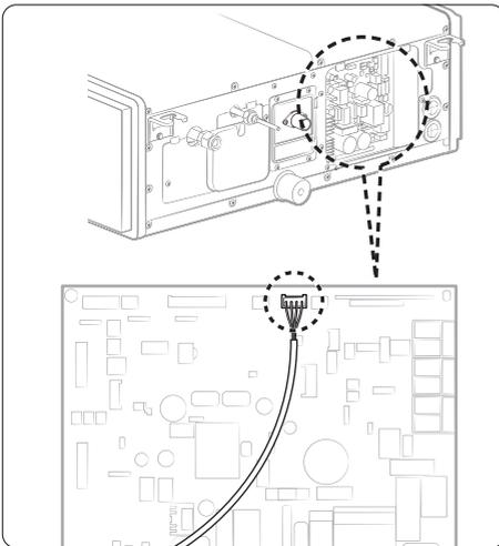
4 Pull out the Wi-Fi wire through the wire hole, and then take out the Wi-Fi module from the back side of the Cover pipe.
