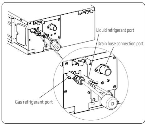
**Step 8 Performing the gas leak test**
