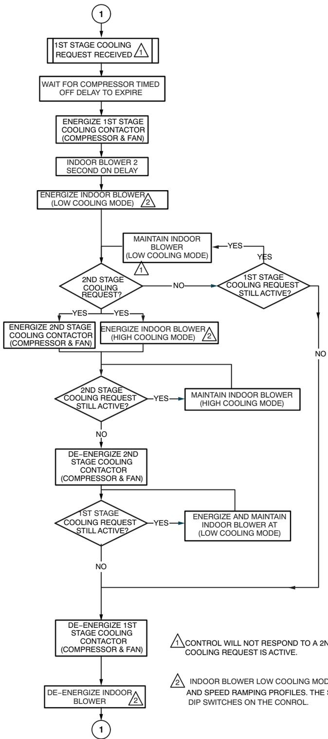
1 CONTROL WILL NOT RESPOND TO A 2ND STAGE COOLING REQUEST UNLESS A 1ST STAGE COOLING REQUEST IS ACTIVE.
