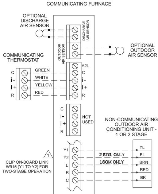
**Communicating Enabled Furnace and Communicating Enabled Outdoor Unit**
