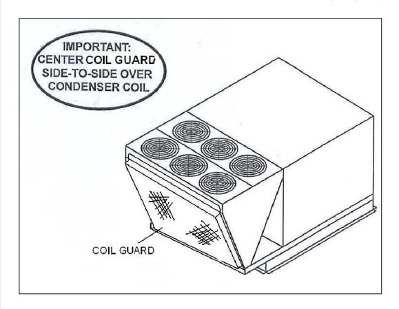
4. SCREW THE SIDE FLANGES OF THE GUARD WITH THE UNIT. TO AVOID COIL DAMAGE, USE ONLY 1/2" SCREWS PROVIDED.
