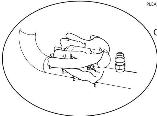
**C** USE A WET RAG TO PROTECT CTXV SENSING BULB WHEN BRAZING SUCTION LINE CONNECTIONS.
