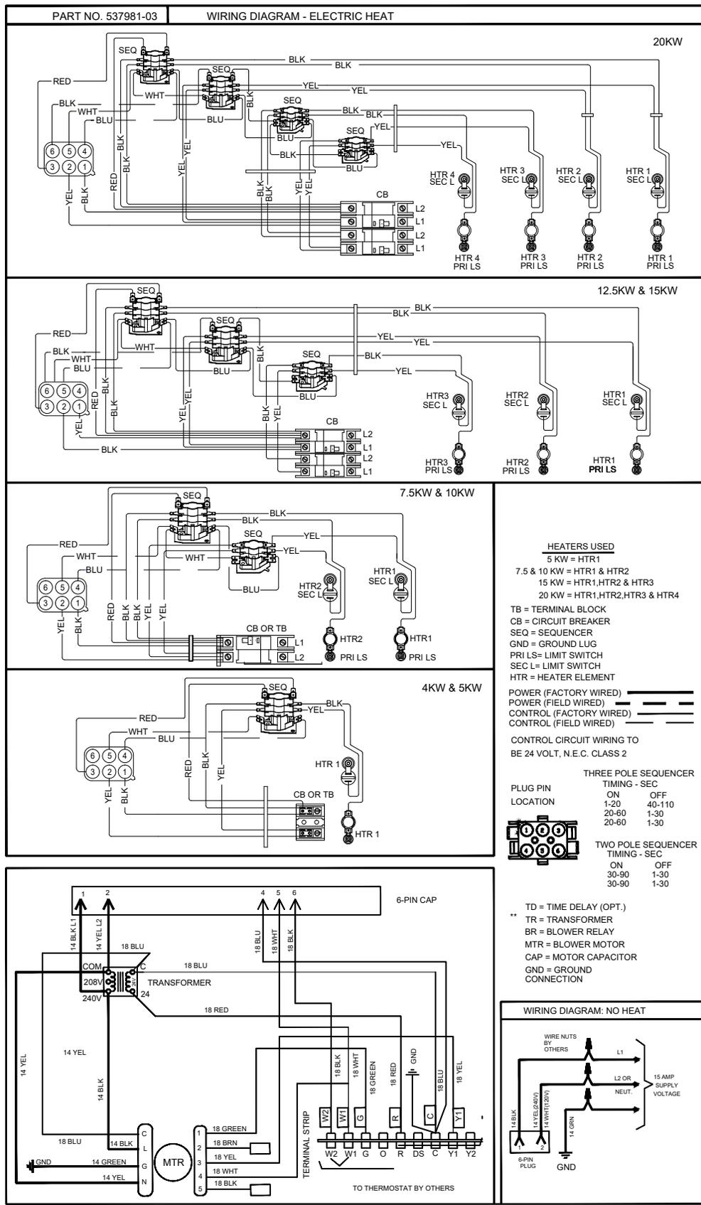
**FIGURE 21. Unit Wiring Diagram – Electric Heat and Air Handler**
