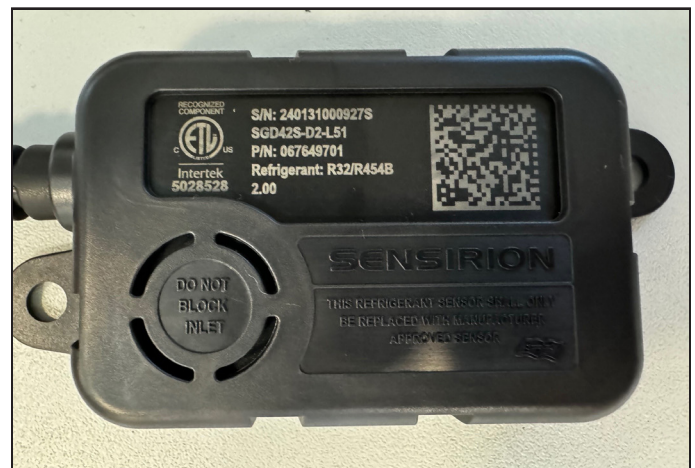
FIGURE 14. Example of Clear, Unobstructed Sensor Inlet
