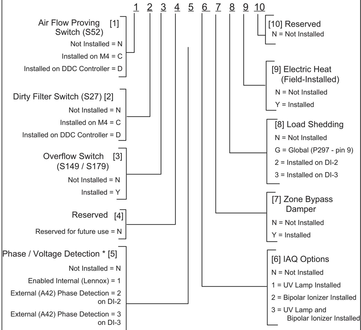
\* When phase detection and voltage monitoring is enabled and wired incorrectly, the system will go into demand hold status and restart after six minutes.
