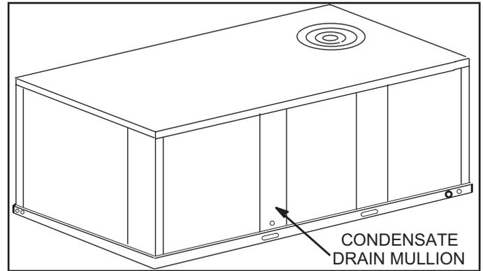
Two hinge screws must be removed in addition to the mullion screws. See FIGURE 6.
