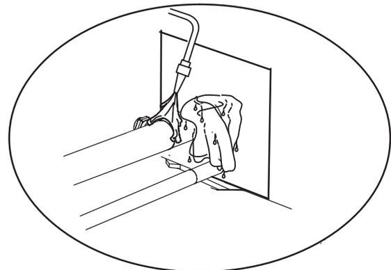
REFER TO INSTRUCTIONS PROVIDED WITH OUTDOOR UNIT FOR LEAK TESTING, EVACUATING AND CHARGING PROCEDURES
