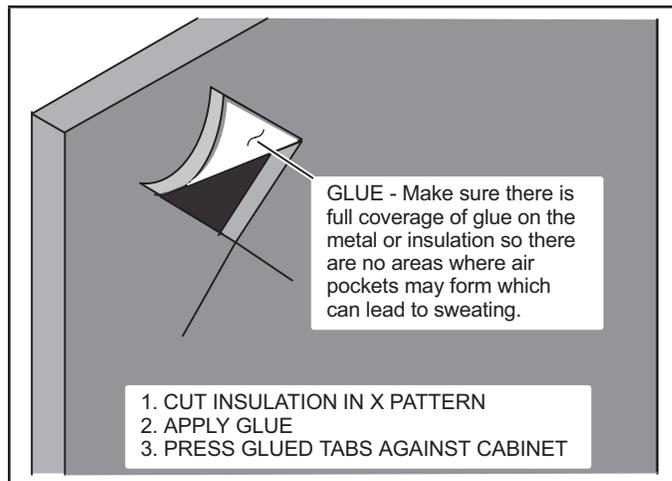
FIGURE 19. Repairing Insulation
