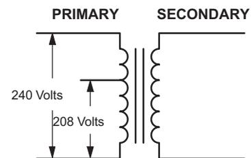
**FIGURE 13. Converting Unit from 240VAC to 208VAC**
