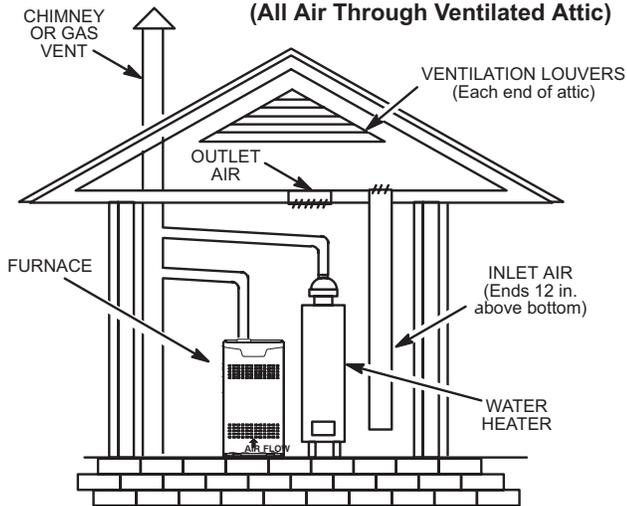
*NOTE-The inlet and outlet air openings shall each have a free area of at least one square inch (645 mm<sup>2</sup>) per 4,000 Btu (1.17 kW) per hour of the total input rating of all equipment in the enclosure.*
