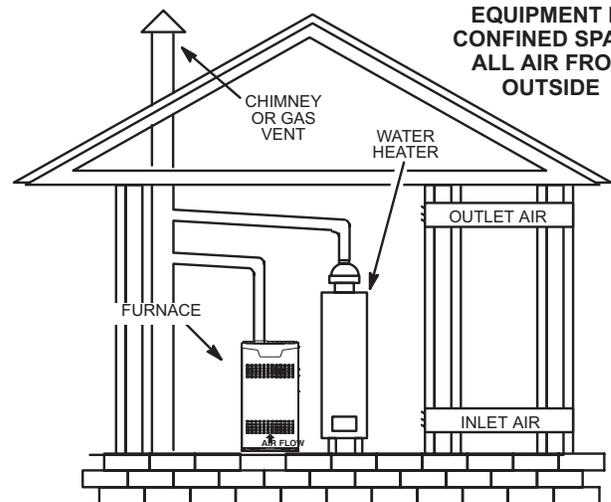
*NOTE - Each air duct opening shall have a free area of at least one square inch (645 mm<sup>2</sup>) per 2,000 Btu (.59 kW) per hour of the total input rating of all equipment in the enclosure. If the equipment room is located against an outside wall and the air openings communicate directly with the outdoors, each opening shall have a free area of at least one square inch (645 mm<sup>2</sup>) per 4,000 Btu (1.17 kW) per hour of the total input rating of all other equipment in the enclosure.*
