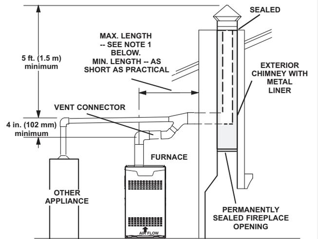
**NOTE 1 -** Refer to the provided venting tables for installations. Refer to the capacity requirements shown in the provided venting tables.
