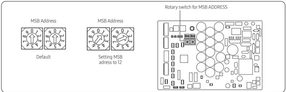
※ V2MSBB12HR model has three PBAs, and V2MSBB08HR & V3MSBB06HR models have two PBAs in the control box.
