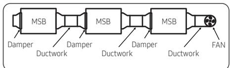
The evacuation channel and the damper must be installed on opposite sides.
