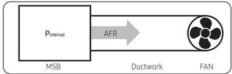
To select the fan of the appropriate specifications, consider the legal requirements and the total pressure drop in the duct system.
