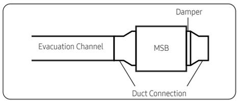
The damper is designed to allow its installation on either side. If you want to reposition the damper, you need to unscrew and disassemble the damper assembly, then unplug the damper motor wire from the connector and move it. Reassemble the damper assembly on the opposite side and plug the damper motor wire back into the nearest PBA.
