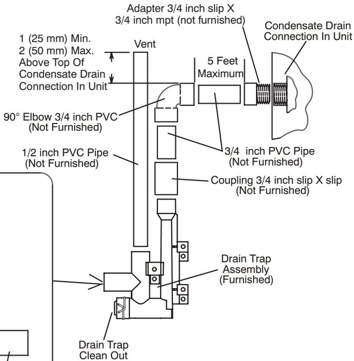
**Drain Trap Assembly with 1/2 inch Piping**
