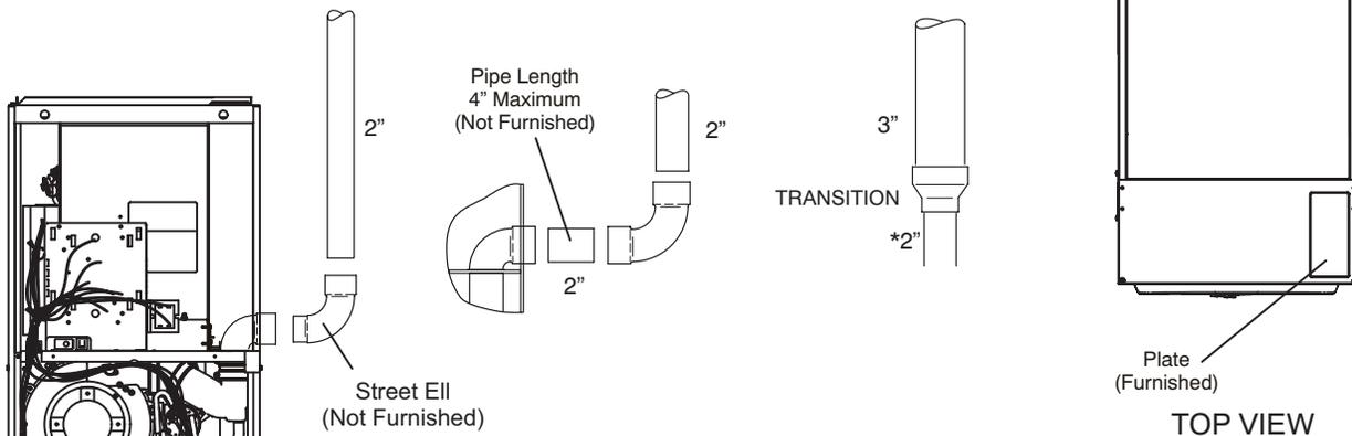
\* When transitioning up in pipe size, use the shortest length of 2" PVC pipe possible.
