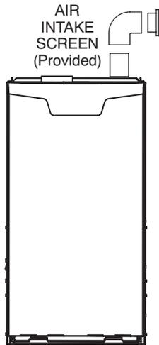
**NOTE** - Air intake screen and elbow may be rotated, so that screen may be positioned to face forward or to either side.
