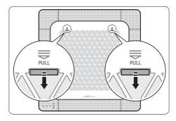
3 Hang the panel on the 2 hooks on the both sides of the indoor unit firmly so that the panel not to fall out.
