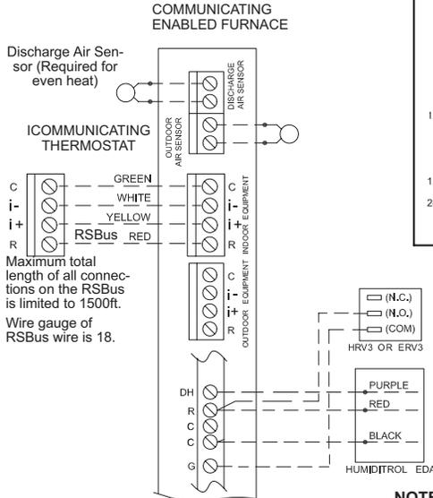
Maximum total length of all connections on the RSBUS is limited to 1500ft. Wire gauge of RSBUS wire is 18.
