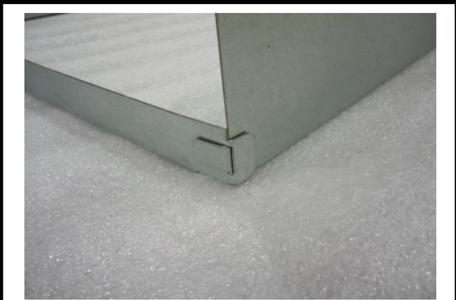
Fig. 6a: Tab Inside Support with Top Rail
