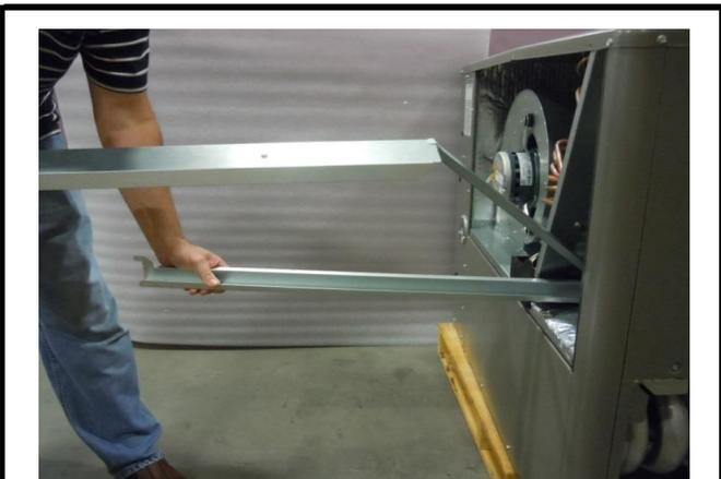
Fig. 7a: Scissor 3-piece assembly into unit
