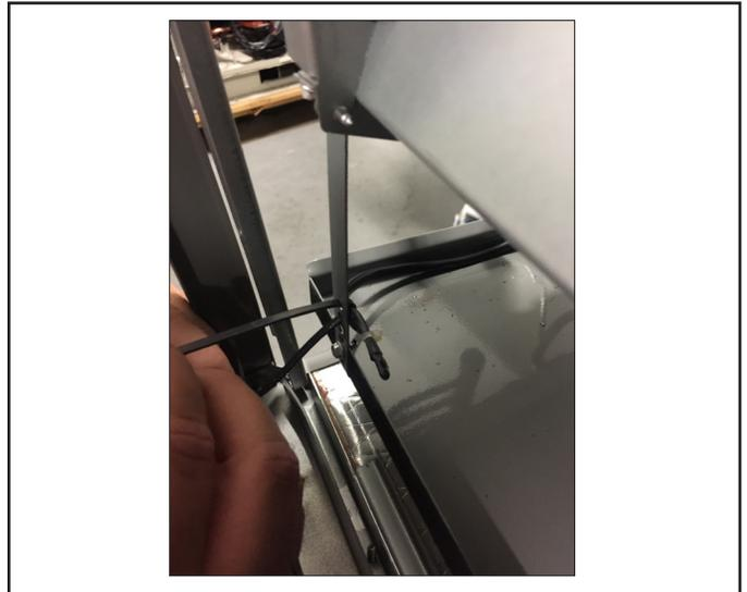
**Figure 12. Relocate T-1 Sensor**
