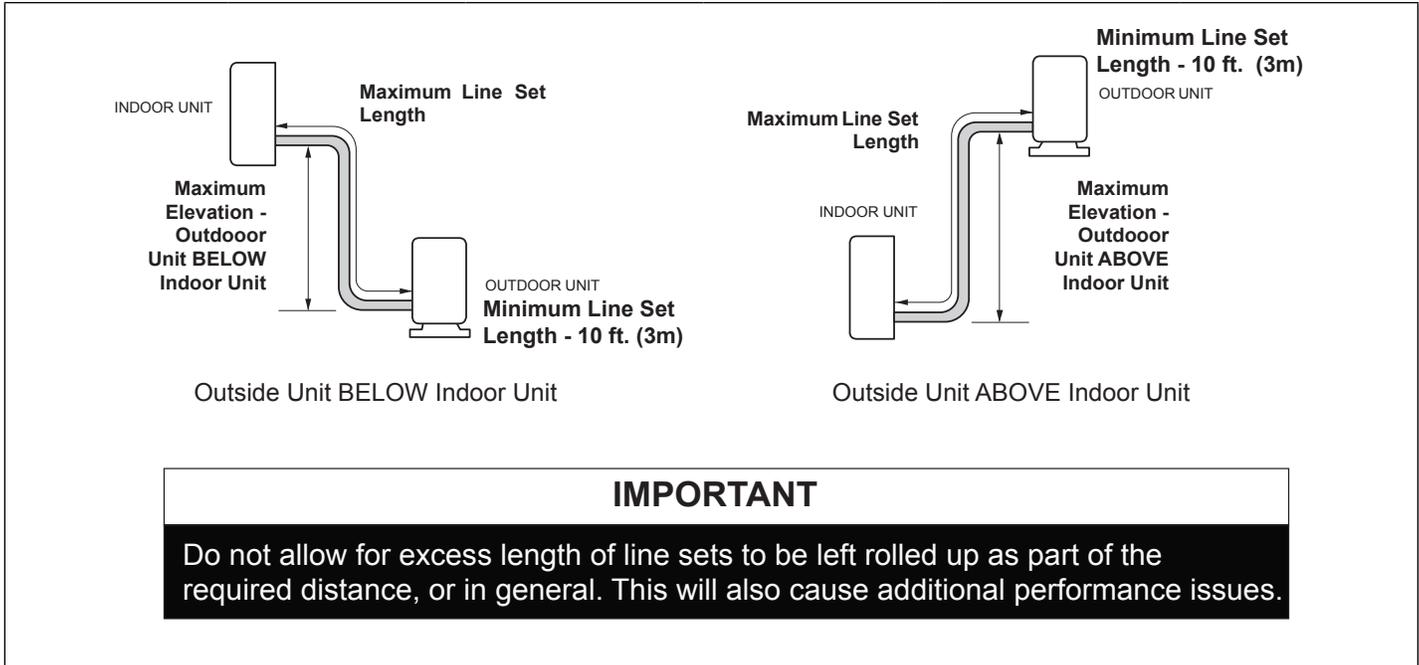
Each system size has a line set length and vertical elevation parameters.
