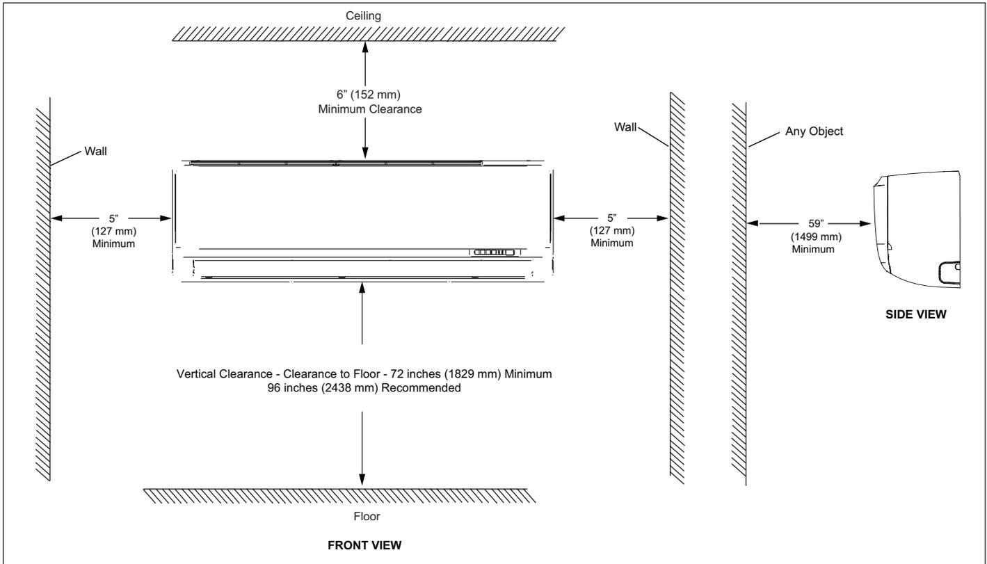
**Figure 6. Indoor Unit Clearances - Inches (mm)**
