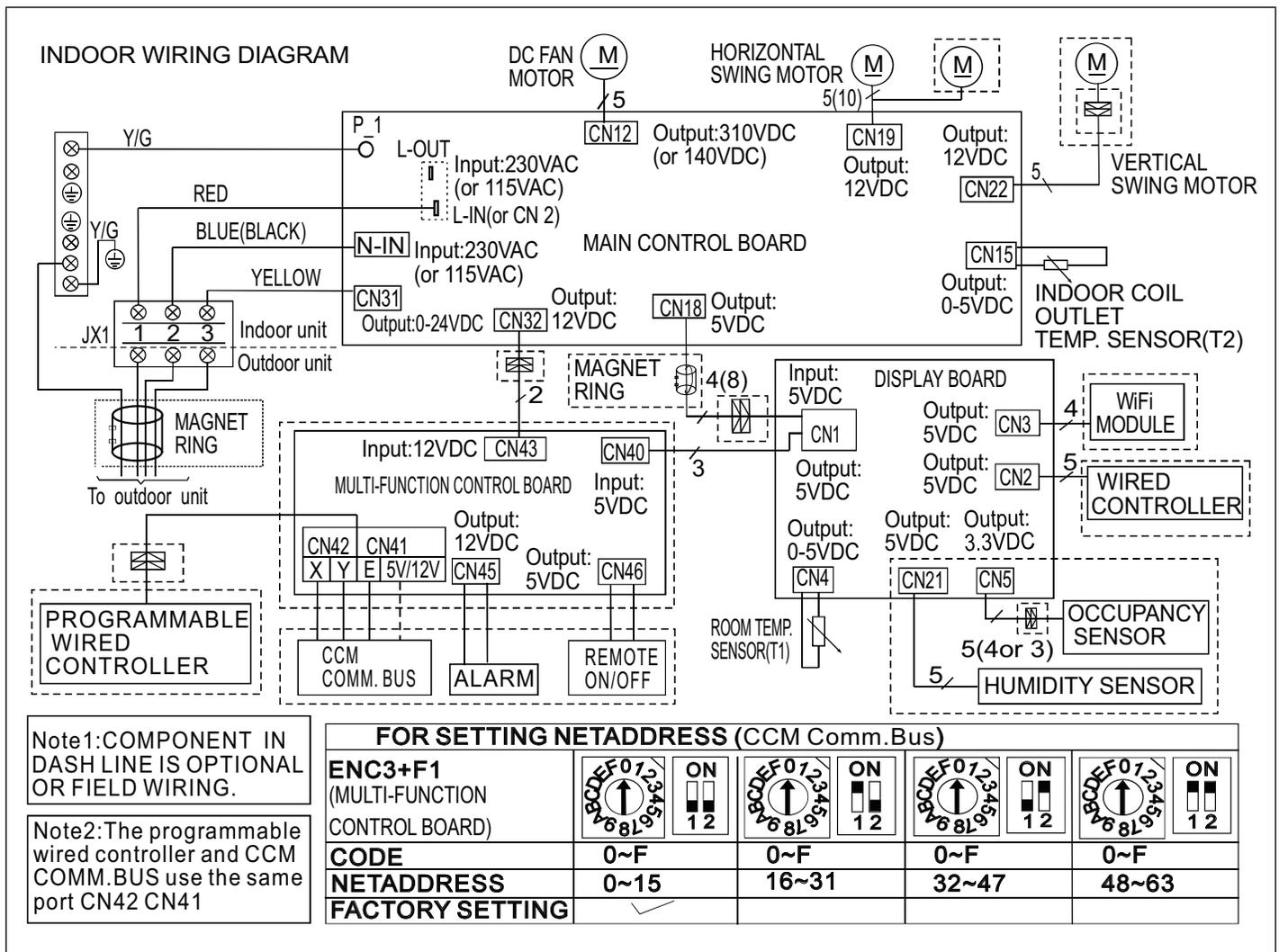
Figure 29. 3WMC036 Indoor Unit Wiring Diagram
