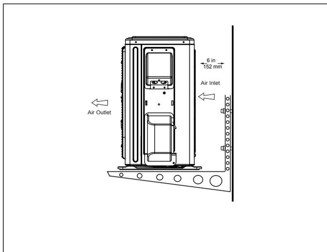
**Figure 23. Securing Outdoor Unit to Brackets**
