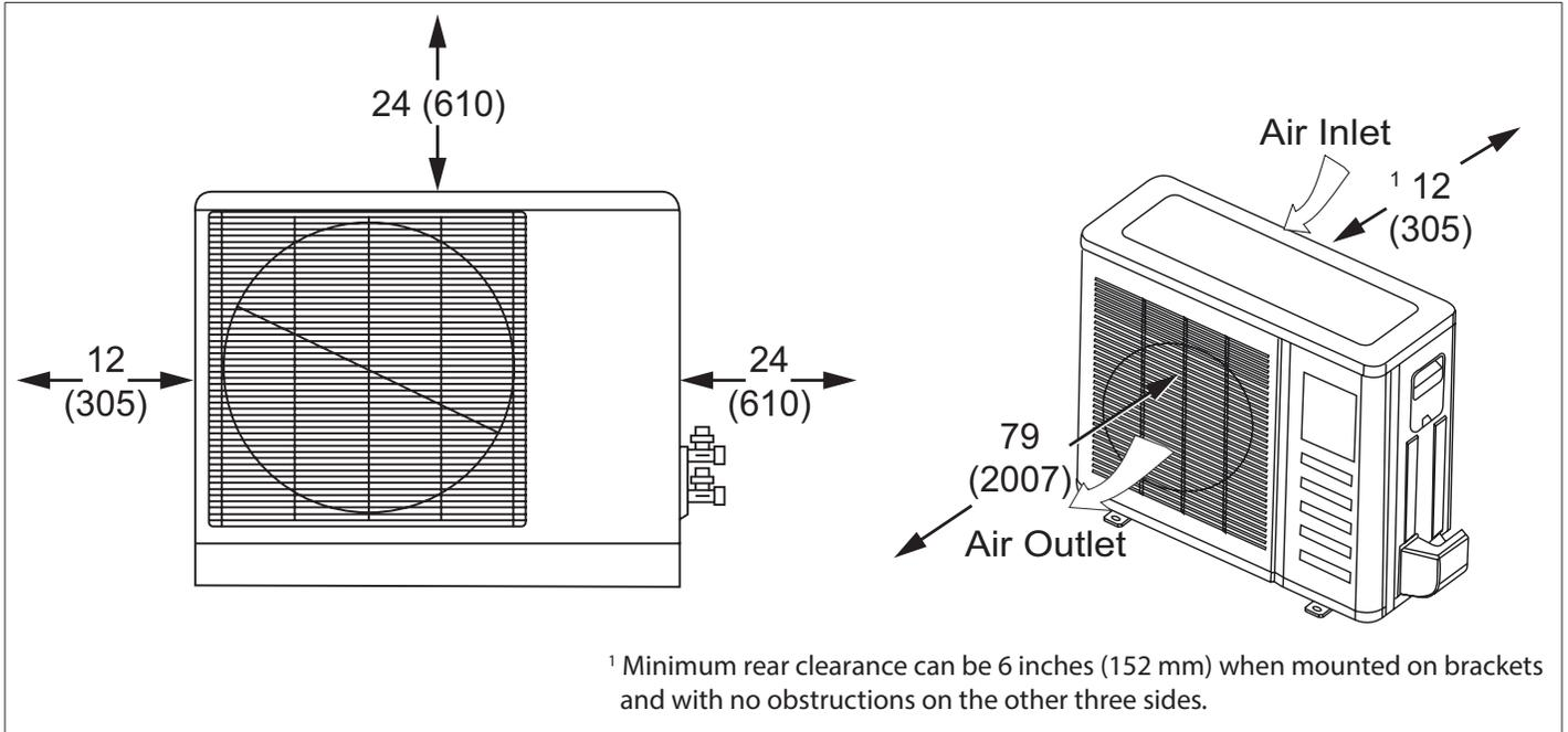
**Figure 5. Outdoor Unit Clearances - Inches (mm)**
