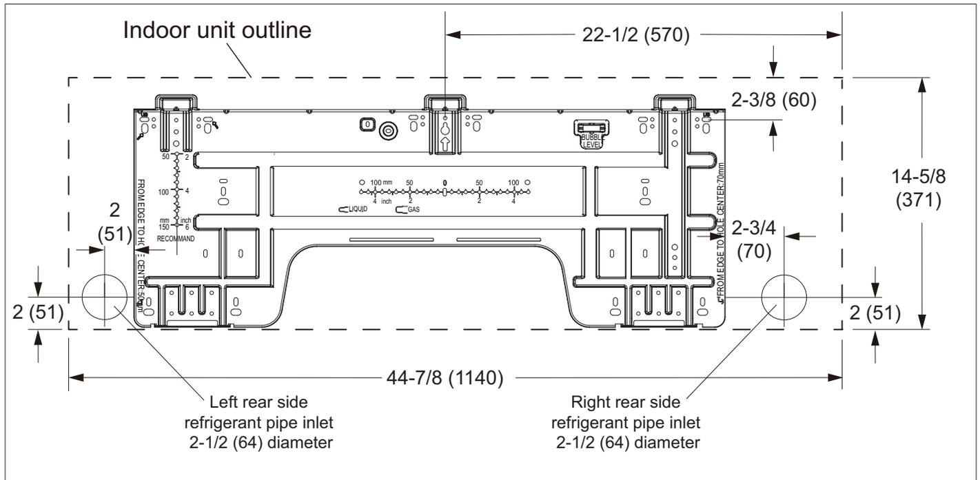
**Figure 4. Indoor Unit Wall Plate Dimensions - Inches (mm)**
