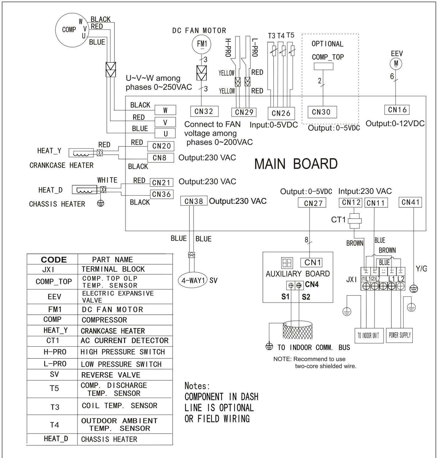
Figure 28. 3PC036 Outdoor Unit Wiring Diagram
