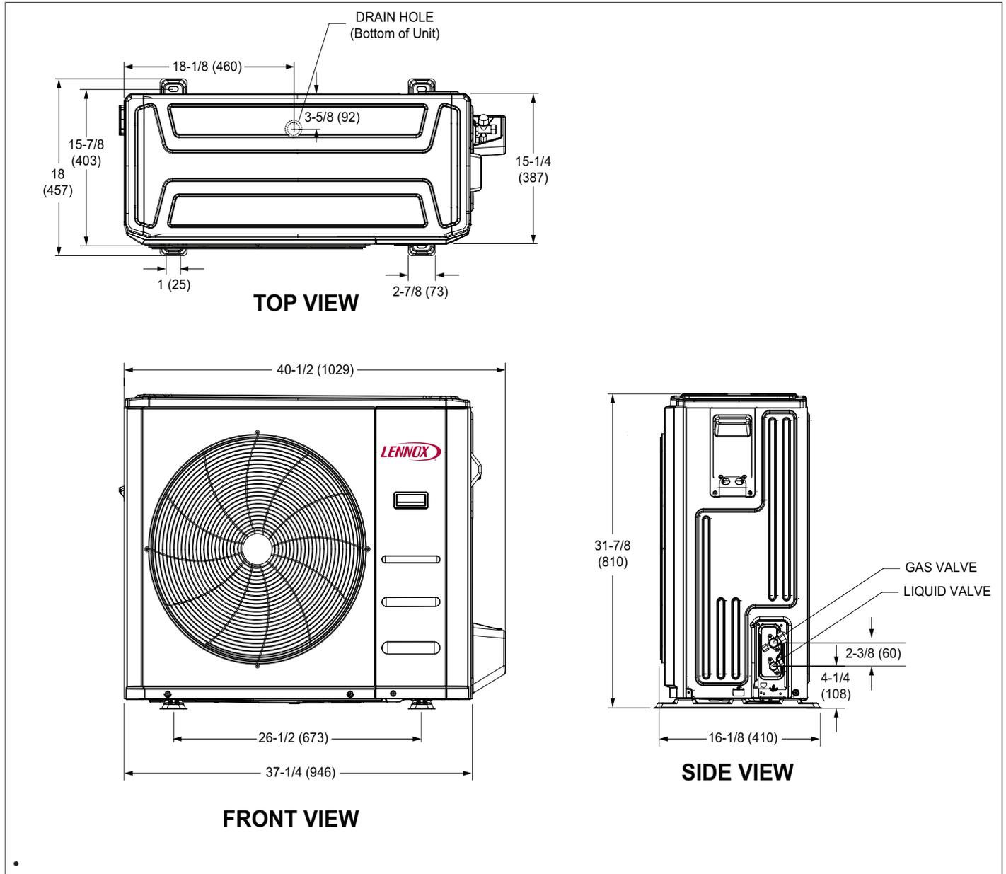
Figure 2. 3PC036S4S-1P Outdoor Unit Dimensions - Inches (mm)
