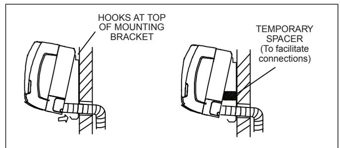
Figure 10. Secure Unit to Wall Mounting Plate
