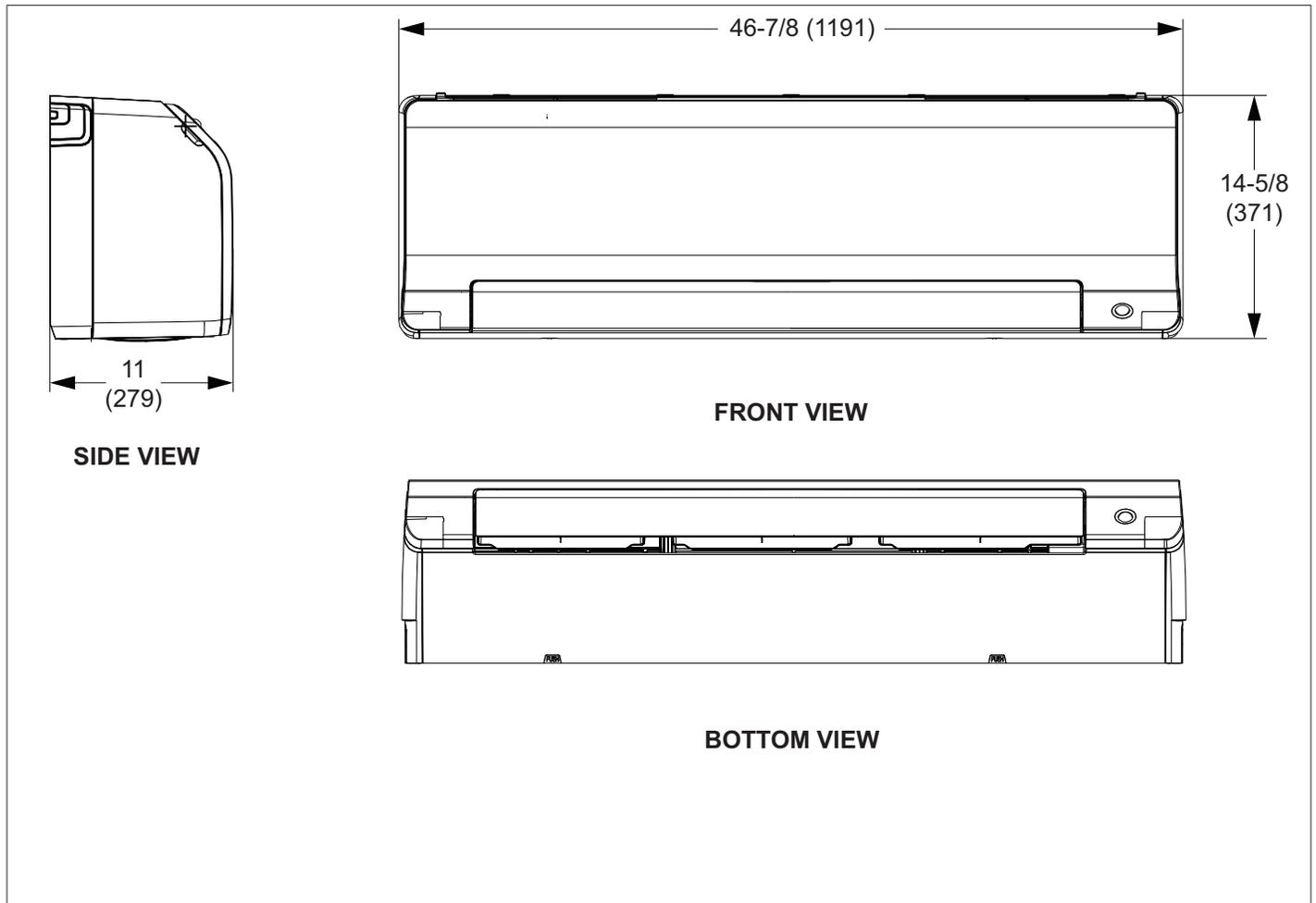
**Figure 3. Indoor Unit Dimensions - Inches (mm)**
