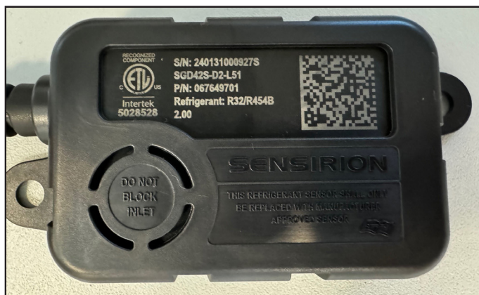
FIGURE 35. Example of Clear, Unobstructed Sensor Inlet
