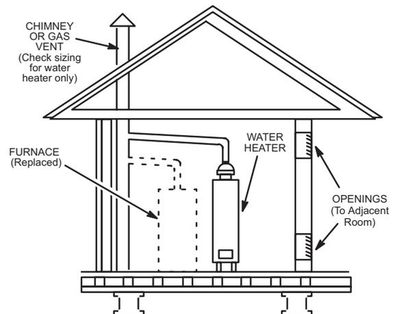
If replacing a furnace which was commonly vented with another gas appliance, the size of the existing vent pipe for that gas appliance must be checked. Without the heat of the original furnace flue products, the existing vent pipe is probably oversized for the single water heater or other appliance. The vent should be checked for proper draw with the remaining appliance.
