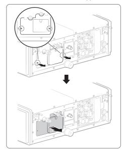
**4** Pull out the Wi-Fi wire through the wire hole, and then take out the Wi-Fi module from the back side of the pipe cover.
