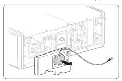
5 Connect the Wi-Fi wire connector through the wire hole .
