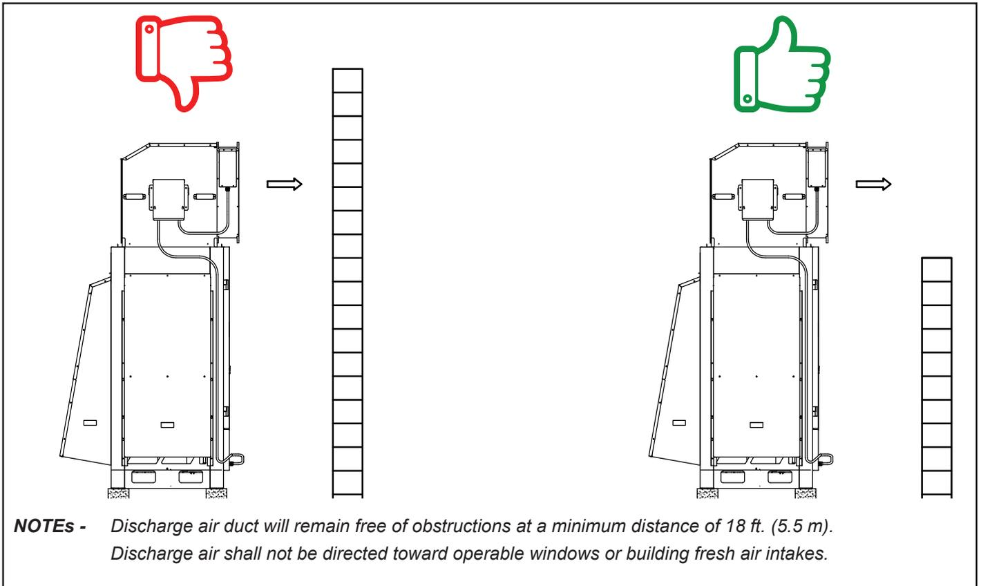
**Figure 2. Direct Hood Discharge Out and Over Enclosure Walls**
