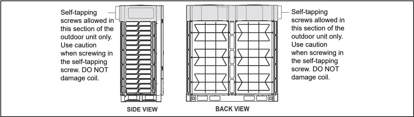
**Figure 10. Field-Made Screw Hole Permitted Locations**
