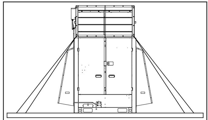
**Figure 7. Secure Unit with Safety Strap (Sides)**
