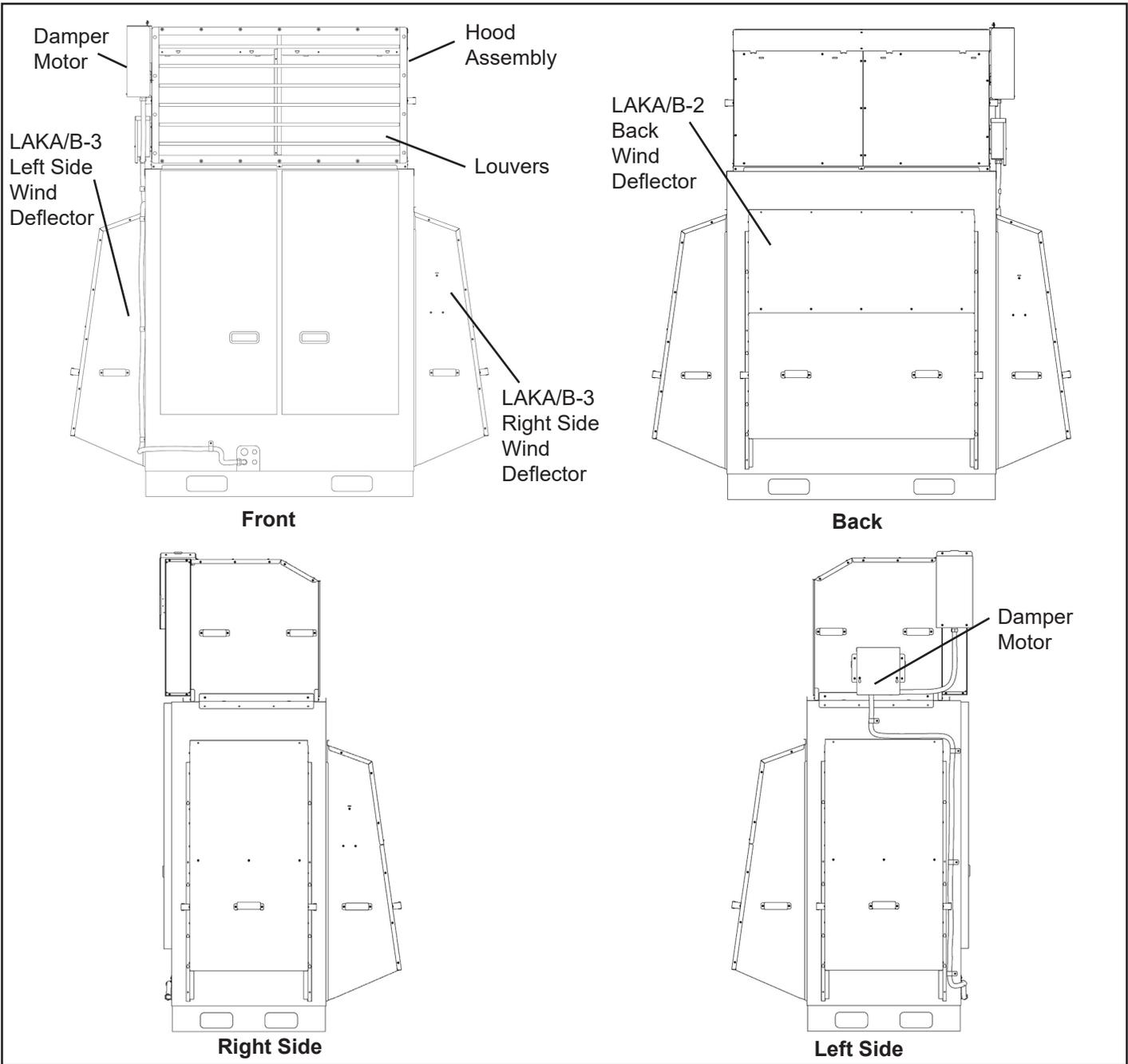
**Figure 11. Low Ambient Kit Installed (All Views)**
