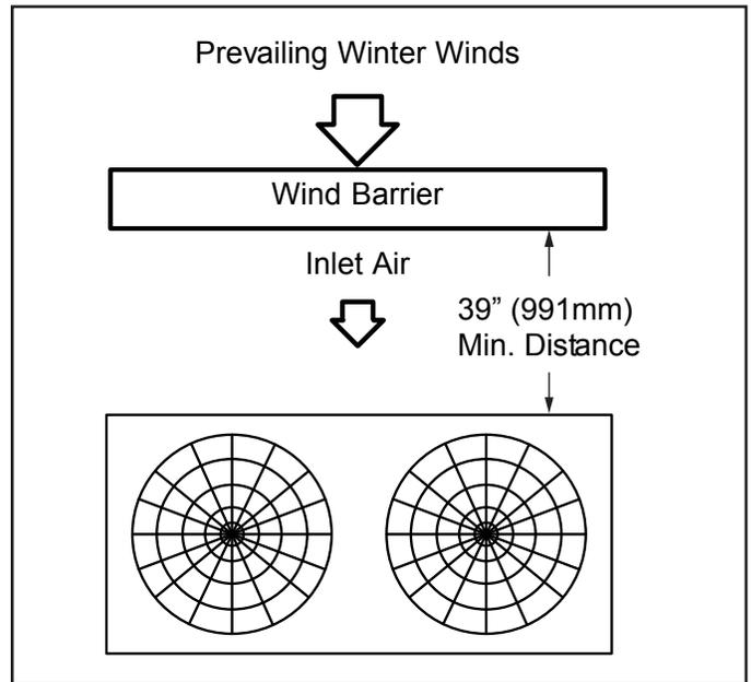
**Figure 1. Prevailing Winds Barrier**
