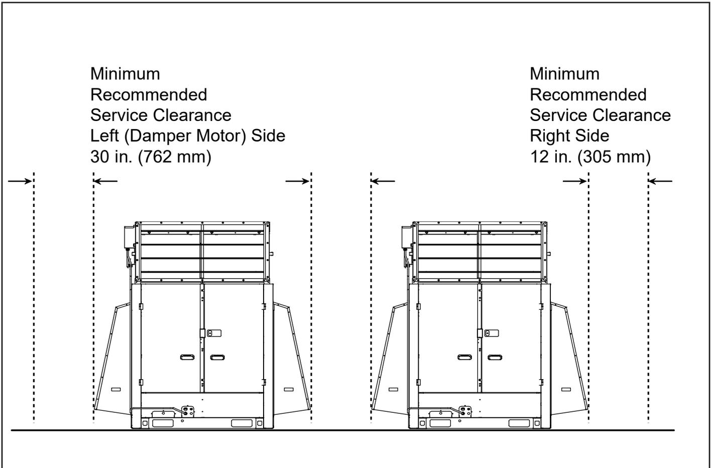
**Figure 3. Distance Between Units with Kit Installed**
