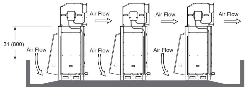
**NOTES -** Discharge air duct will remain free of obstructions at a minimum distance of 18 ft. (5.5 m).
