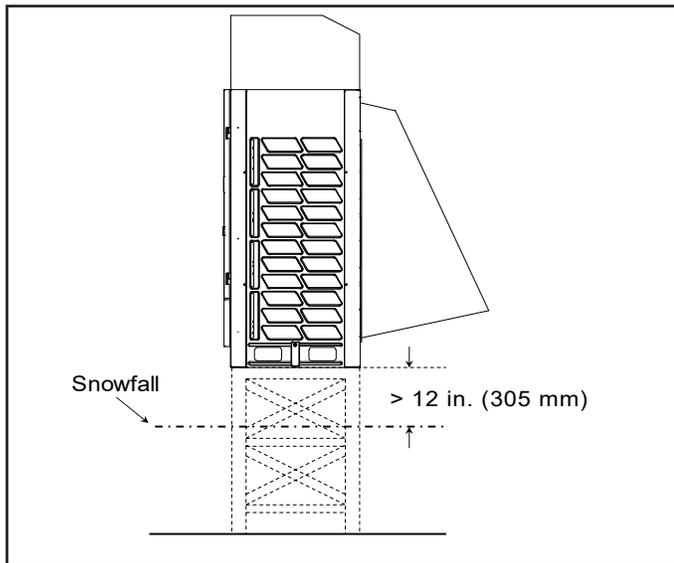
**Figure 4. Elevate Unit Above Snow Level**
