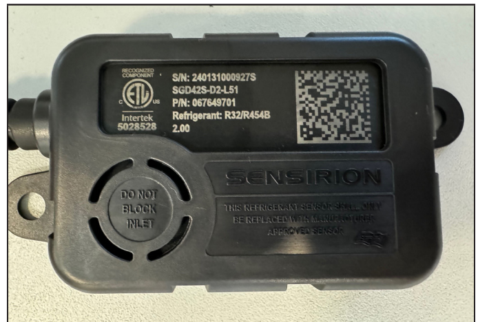
FIGURE 36. Example of Clear, Unobstructed Sensor Inlet
