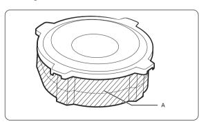
Insulate the end of the pipe and some curved area by using separate insulator.
