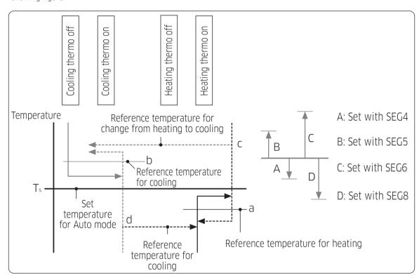
The mode change between the Cool and Heat modes is made only when the thermo off state is maintained for the period of time set with SEG9.
