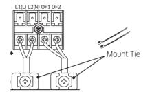
As shown in the figure, connect the wire from the outdoor unit to the kit terminal block and then fix the wire onto the mount tie by using the provided cable tie.
