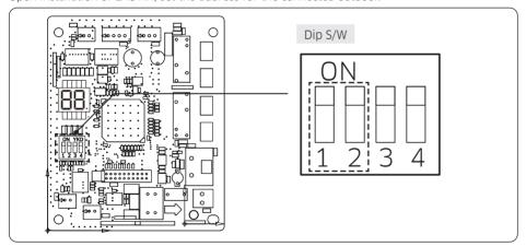
• Prior to power supply to the outdoor unit, set the switches. When address recognition is impossible after power supply, press the Reset button (K3 switch) on the outdoor unit.
