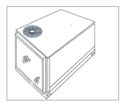
5. REPEAT THE PROCESS FOR THE MEDIUM AND LARGE GUARDS. TO AVOID COIL DAMAGE, USE ONLY 1/2" SCREWS PROVIDED.
