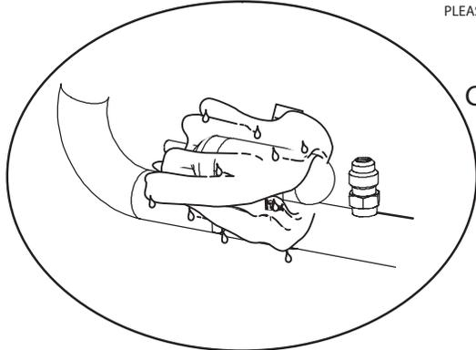
**C** USE A WET RAG TO PROTECT CTX SENSING BULB WHEN BRAZING SUCTION LINE CONNECTIONS.
