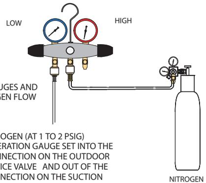
FLOW REGULATED NITROGEN (AT 1 TO 2 PSIG) THROUGH THE REFRIGERATION GAUGE SET INTO THE VALVE STEM PORT CONNECTION ON THE OUTDOOR UNIT LIQUID LINE SERVICE VALVE AND OUT OF THE VALVE STEM PORT CONNECTION ON THE SUCTION SERVICE VALVE.
