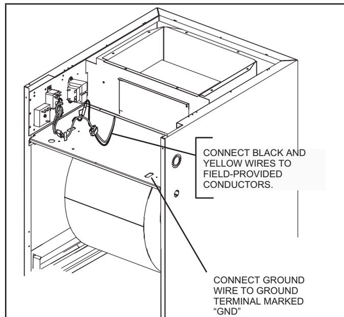
FIGURE 25. Making Electrical Connections
