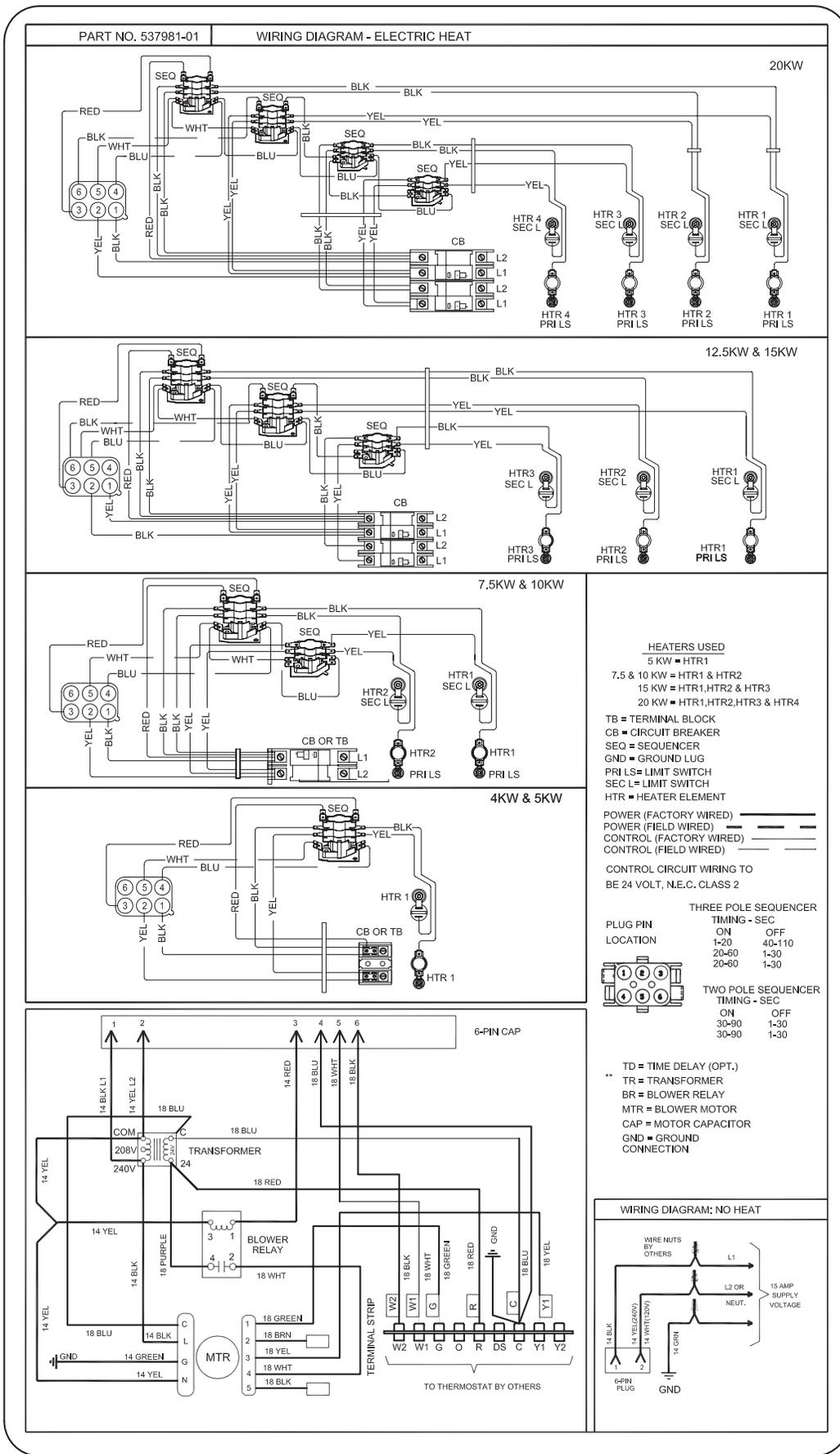
**FIGURE 29. Unit Wiring Diagram – Electric Heat and Air Handler**
