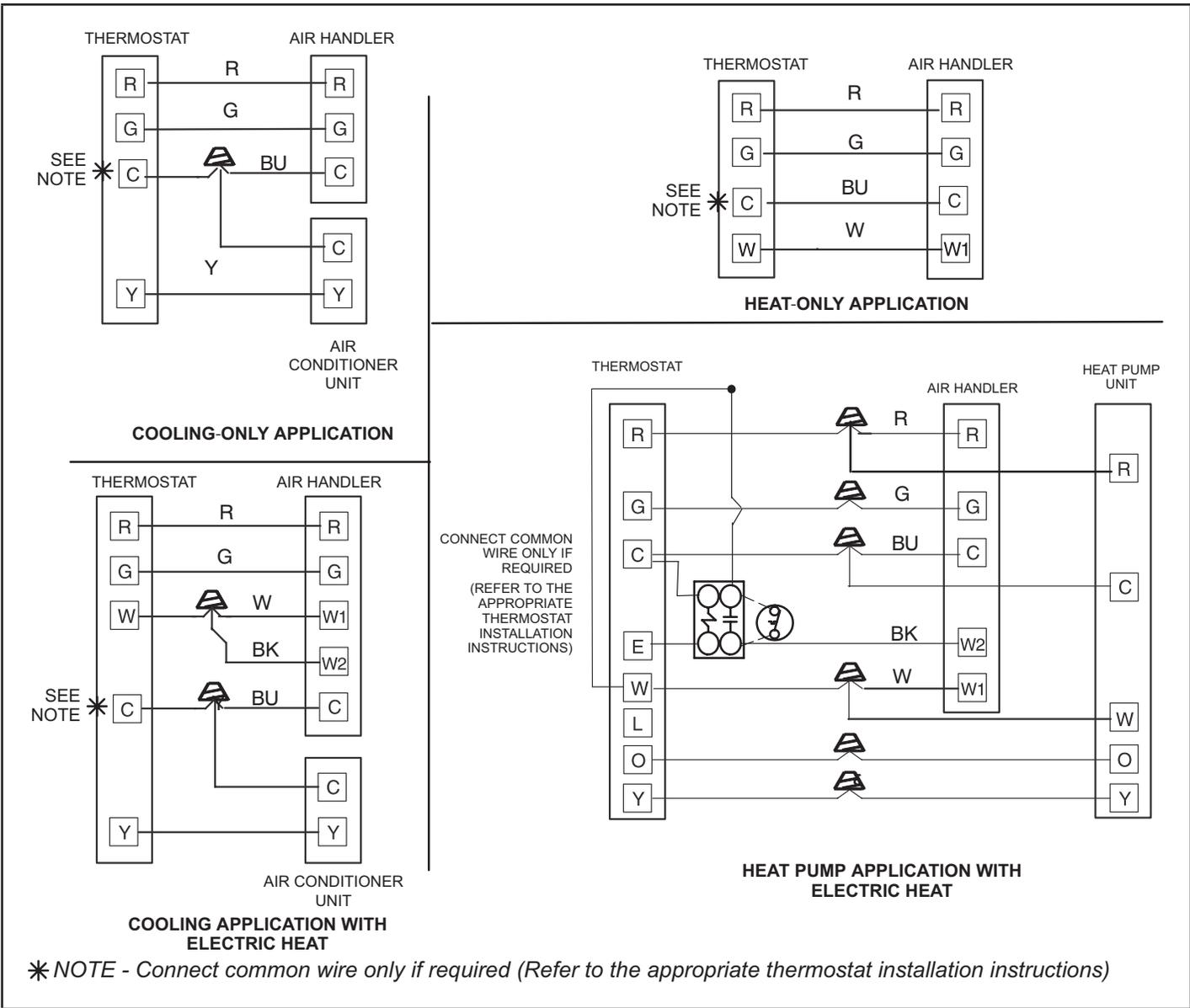
**FIGURE 26. Low Voltage Connections (3-Speed PSC Motor) – Field Wiring**
