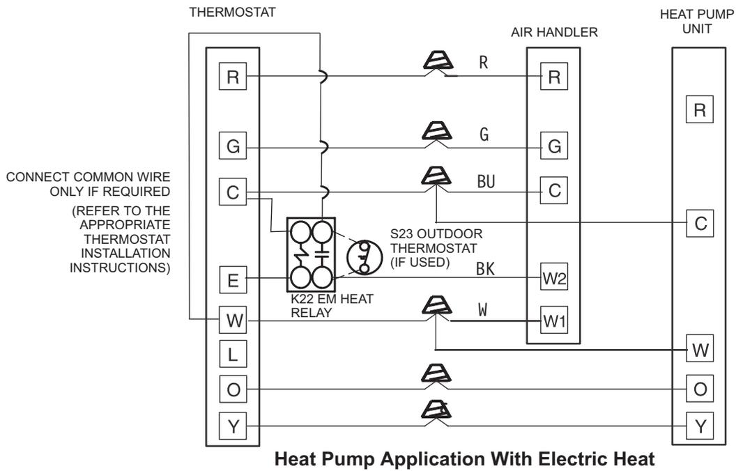
**FIGURE 27. Low Voltage Field Wiring Electric Heat**
