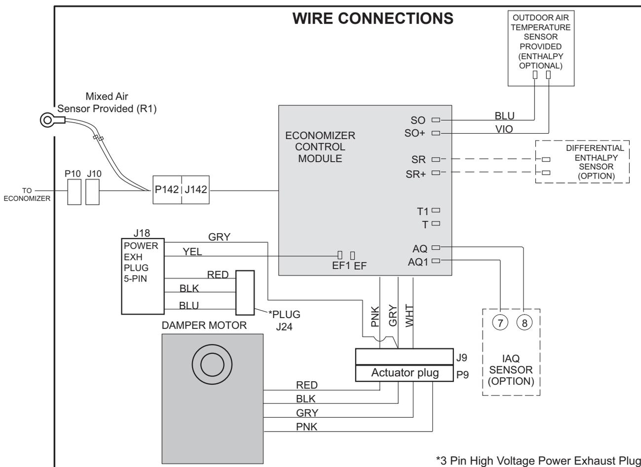
Figure 5 - Wiring Detail
