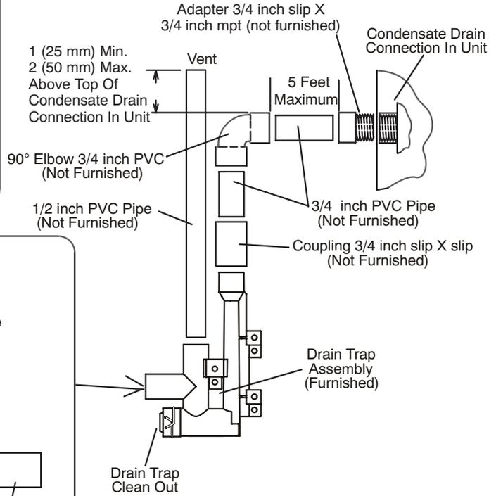
Drain Trap Assembly with 1/2 inch Piping
