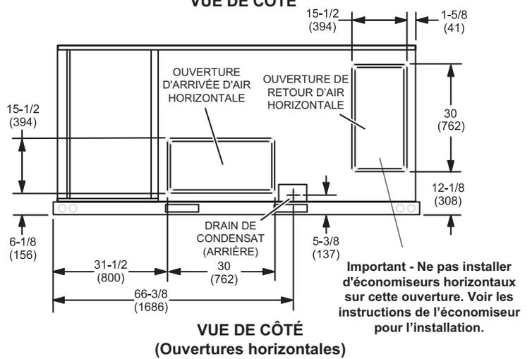
**LHT/LDT152H DIMENSIONS - SECTION DE CHAUFFAGE AU GAZ ILLUSTRÉE**
