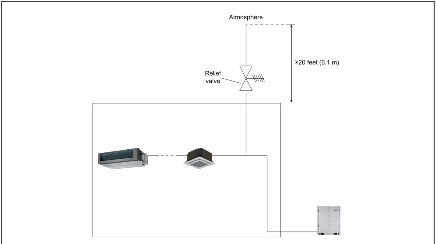
Figure 22. Refrigerant Discharge
