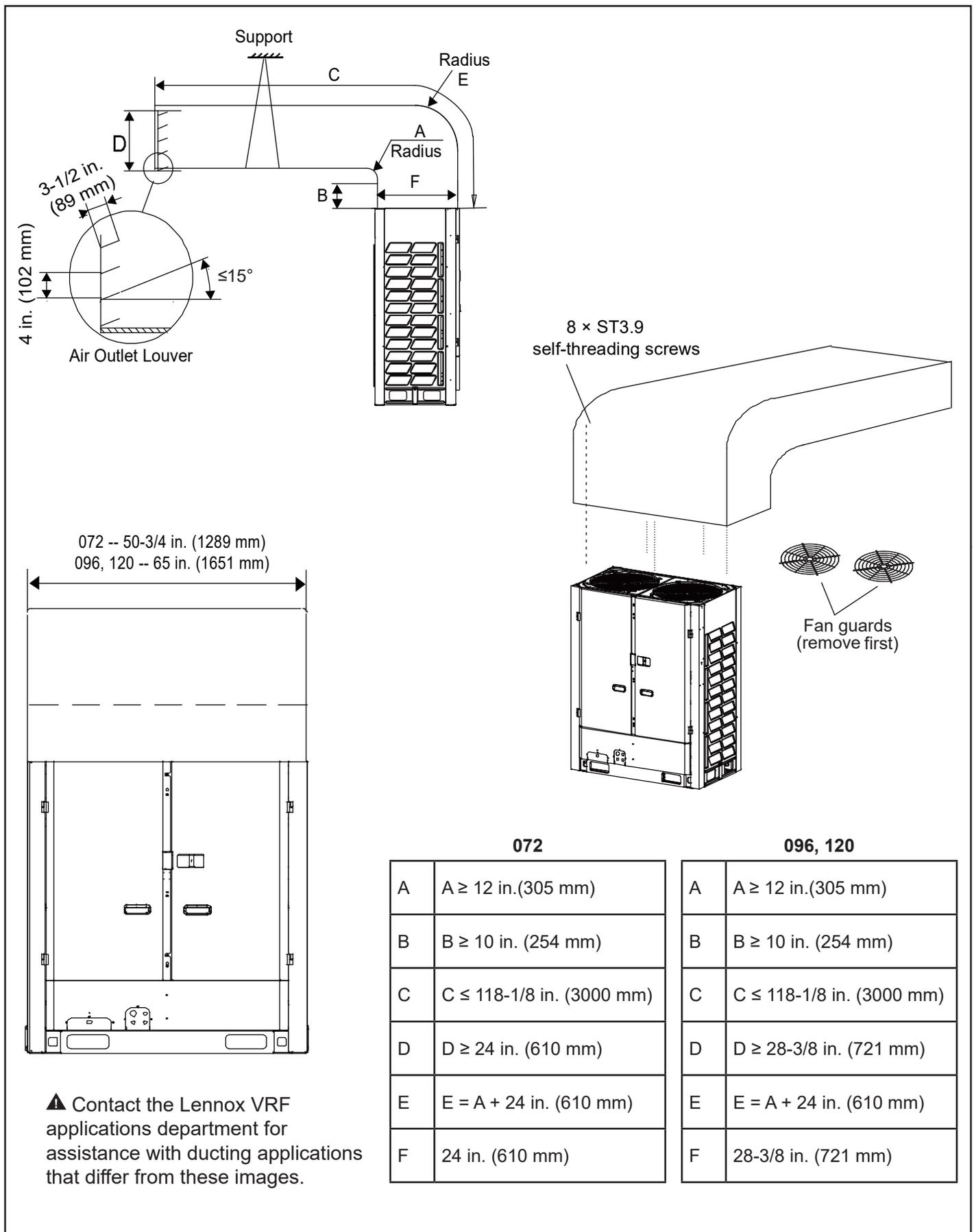
**Figure 10. Air Discharge Duct
