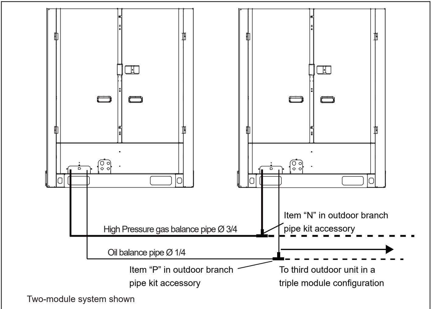
**Figure 25. Connective Piping Sizes for Manifolded Outdoor Units**
