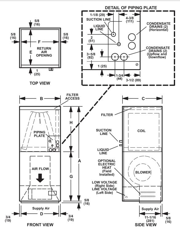
**Note** – Units are shipped in one piece but may be disassembled into two separate sections for ease of installation.
