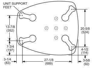
018 TO 036 BASE SECTION 042 TO 060 BASE SECTION (Small Base) (Medium Base)
