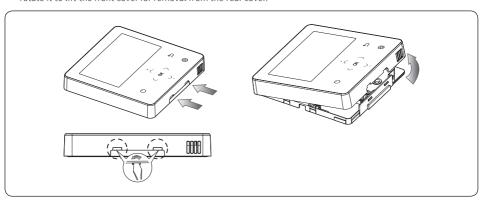
2 Arrange the power cable and the communication cable so that they fit in the housing along the edges of the rear cover.
