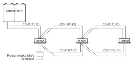
Using One programmable wired controller to control indoor units connected to different outdoor unit
