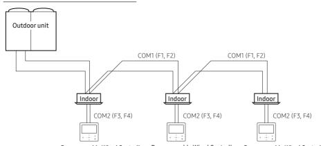
Programmable Wired Controller Programmable Wired Controller Programmable Wired Controller
